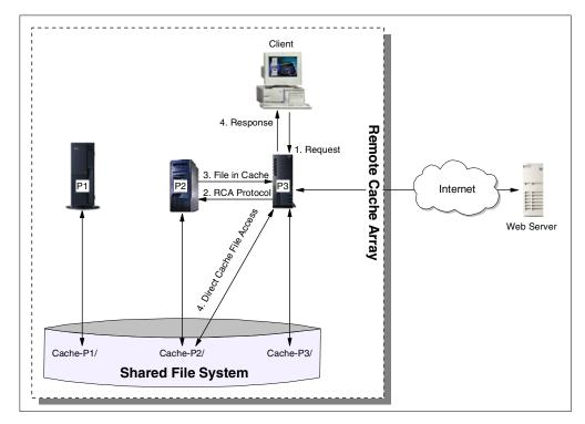
The following diagram shows a graphical representation of an RCA flow:
