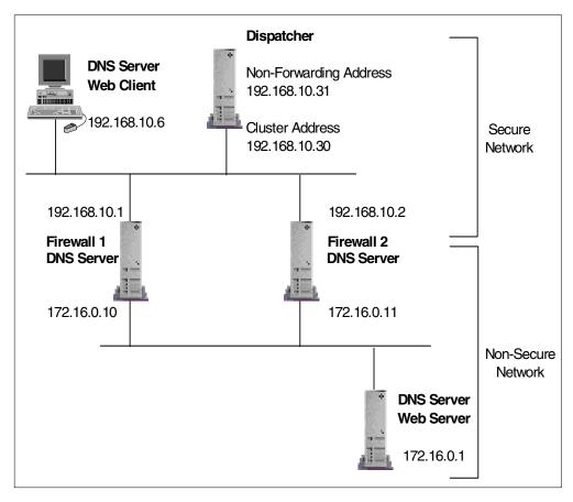
Figure 230. Firewall Load-Balancing Network Environment
