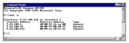
Figure 165. arp -a Associates the MAC Address to an IP Address
