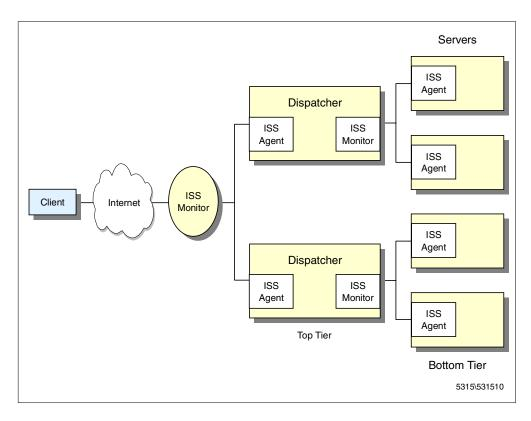
Figure 11. Two-Tiered ISS and Dispatcher Configuration
