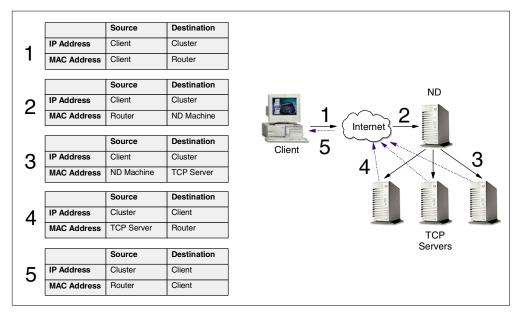
Figure 73. The Flow of the IP Packets
