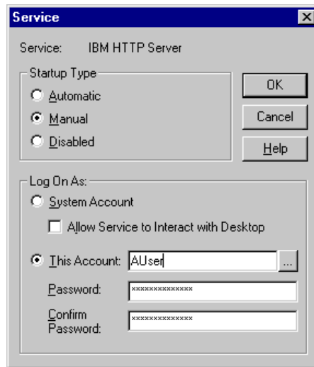
Figure 18. Specifying IBM HTTP Server to Manually Start Up Using a Specific Account
