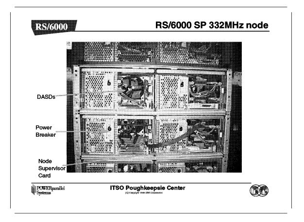
In this front view photograph of RS/6000 SP 332MHz wide node, you can see the DASDs, the node supervisor card, and the power breakers.
