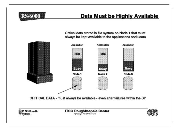
A common requirement is to have critical data on a system that is kept highly available. Solutions do exist to provide this today with NFS, but they have limitations.
