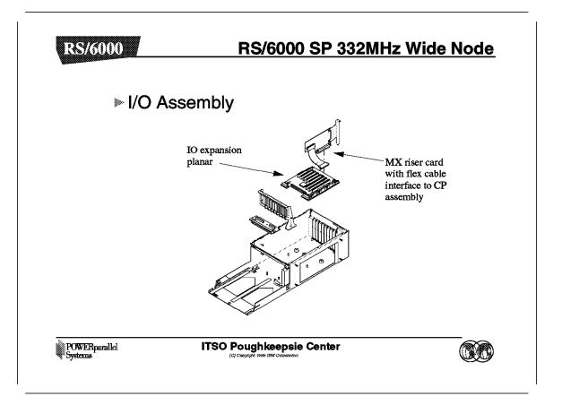
The SMP wide node is composed of a CPU assembly and an I/O assembly. The I/O assembly has an MX riser card, with a flex cable interface to be connected to the CPU assembly.
