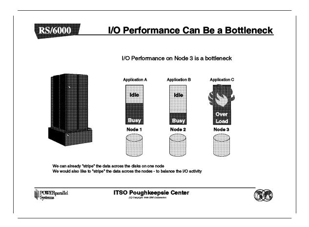
In this example, our application results in a lot of heavy I/O to Node 3. As a result, Node 3 becomes overloaded.
