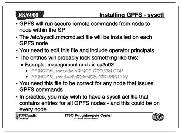
GPFS will not work without sysctl. Check carefully that sysctl is configured and working properly before going any further.
