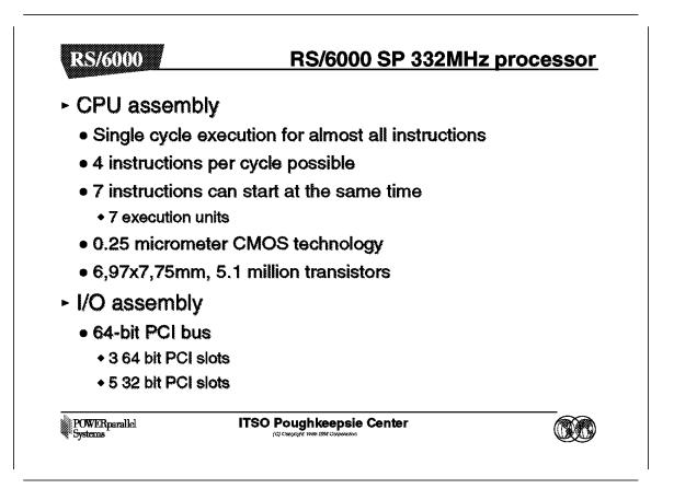
The RS/6000 SP 332MHz SMP nodes are comprised of modular components. Both SMP thin nodes and SMP wide nodes have a CPU assembly which contains a node supervisor, two to four CPUs, one TB3MX slot and two PCI slots.
