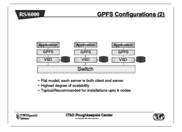
In this example, all nodes are VSD servers and also run the applications. Such a solution would be acceptable for a parallel application that has the same performance requirements across the nodes and exhibits a balanced workload.
