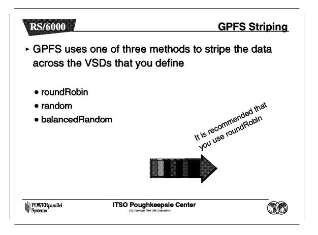
A number of options for GPFS striping exist but the default method, roundRobin, should be the method that you normally use. This is the default selected by GPFS.
