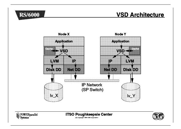
This diagram shows the structure that allows VSD to gain access to remote disks within the SP system.
