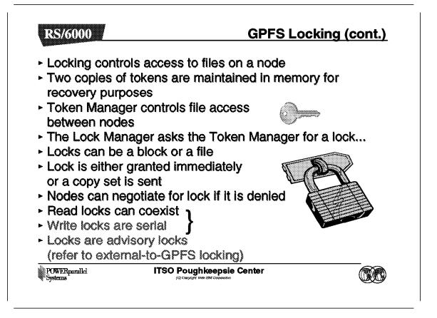
Locking controls access to files from a process point of view on any particular node within the GPFS pool. Two copies of the locks are maintained within the GPFS system to allow for recovery in the event of failure. A Lock Manager runs on each node for the purpose of controlling locking on that node.
