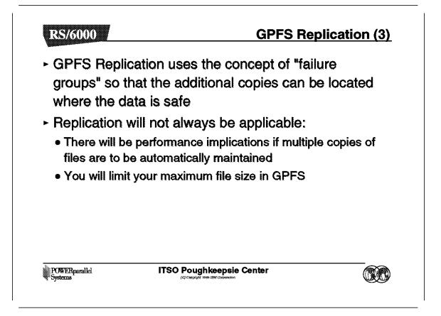
It would not make sense to have another copy of the data and put it on the same disk, or even on a disk attached to the same node, as there would be occasions when we could not get to the extra copy.
