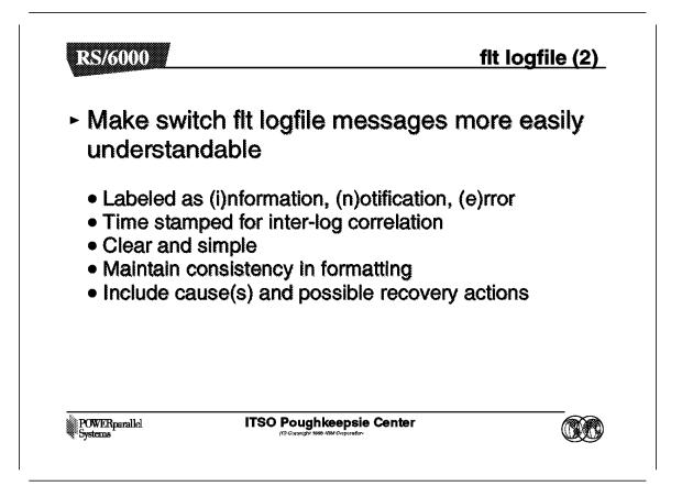
The messages generated for the flt file are modified to include a severity field. Three levels of severity are used:
