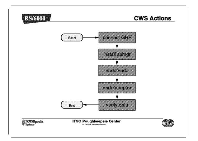
The first CWS action is to connect the RS/6000 SP to the GRF. This includes connecting the SP Switch cable, the GRF administrative Ethernet, and the GRF grounding cable.
