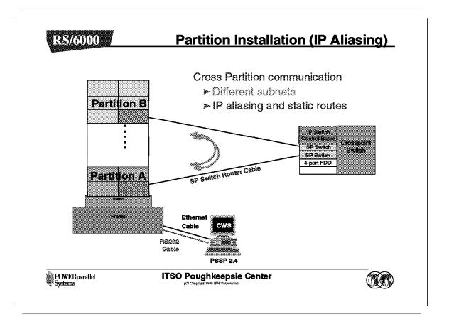
Partitions in the RS/6000 SP are separate networks to the system. Therefore, they should use different subnet masks; this is a requirement when we want them to talk to each other through a single GRF. When both partitions are in the same subnet, the routing table on the GRF will only register one of the routes to the RS/6000 SP. Thus, one of the partitions is not reachable through the GRF.
