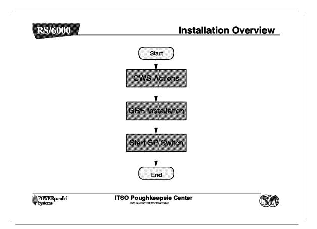
The installation of the dependent node in the RS/6000 SP involves these three steps:
