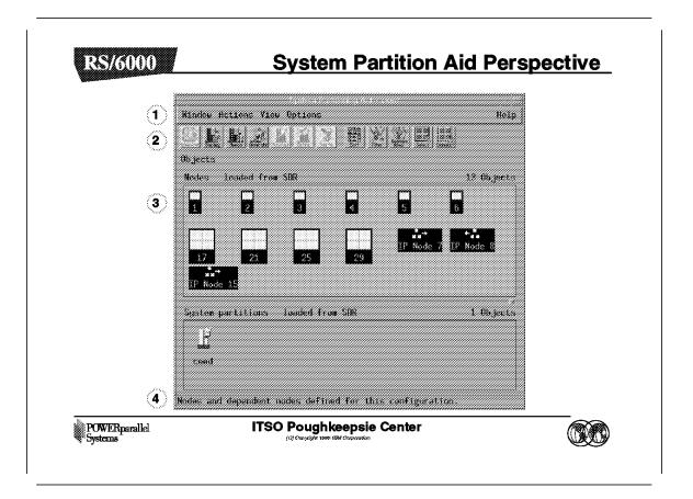
The System Partition Aid Perspective window has two panes, the Nodes pane and the System partitions pane. The Nodes pane (3) in this figure shows the Icon view. Notice that the IP Nodes are displayed after all the standard RS/6000 SP nodes. Also, the node numbers of the IP Nodes are listed below their icons.
