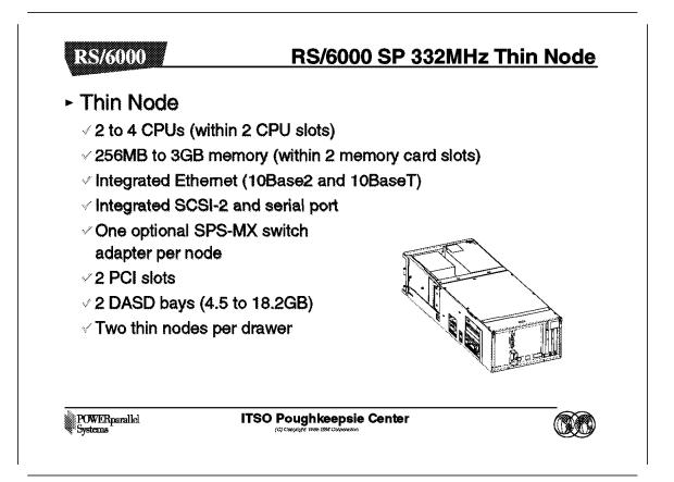
Thin nodes are now available in both a symmetric multiprocessing (SMP) configuration and in the previous uniprocessor configuration. All RS/6000 SP 332MHz SMP thin nodes have Peripheral Component Interconnect (PCI) architecture.
