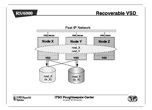
An optional addition that can be used with VSD is Recoverable VSD (RVSD). RVSD is a separate Licensed Program Product (LPP). It is not part of PSSP. It is normally used in conjunction with twin-tailed disks to give high availability for a volume group and the associated VSDs. It is required for GPFS.
