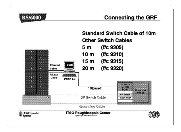
The GRF, when ordered with the SP Switch router adapter, comes with two cables: a 10 meter SP Switch cable, and a 10 meter grounding cable.
