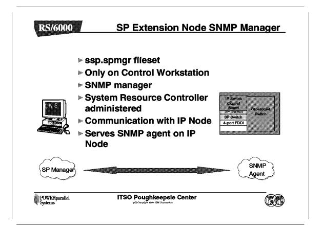
The SP Extension Node SNMP Manager is contained in the ssp.spmgr fileset of PSSP. This fileset must be installed on the Control Workstation in order for the GRF to function as an extension node.
