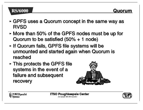
Quorum is used by GPFS to make sure that no unexpected actions occur during a failure within the SP system.
