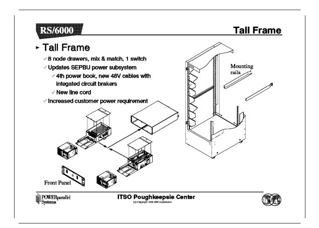
The most noticeable difference between the new and old tall frames is a reduction in height. The new tall frames are now 1.93 meters high, while the older frames are 2.01 meters high.
