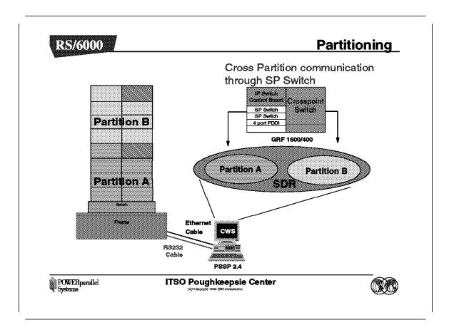
This figure shows a single-frame RS/6000 SP broken into two partitions, Partition A and Partition B. Each partition has seven standard RS/6000 SP nodes and one dependent node. Only seven nodes are allowed in each partition, as a single-frame RS/6000 SP has only 16 SP Switch ports, and two of them are used for the SP Switch router adapter, one for each partition.
