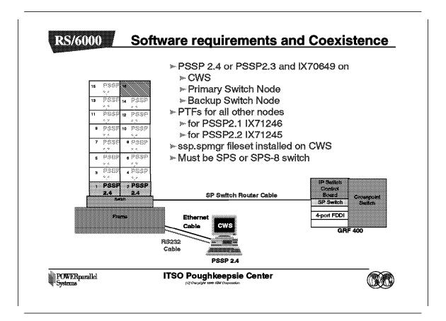
This figure shows a single-frame RS/6000 SP in a single partition with a connection to the GRF. Nodes 1 and 2 are installed with PSSP 2.4. The other nodes are installed with any other version of PSSP that can coexist with PSSP 2.4 to represent coexistence. Also, note that Node 16 is empty, because the SP Switch port for this node is used by the SP Switch router adapter in the GRF.
