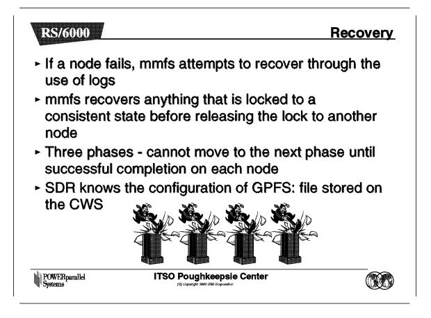
Whenever a node boots, it checks the two GPFS files that are stored in the SDR to see if configuration changes were applied to the GPFS configuration while the node was down. If this is the case, the changes will be applied to the node at that time.
