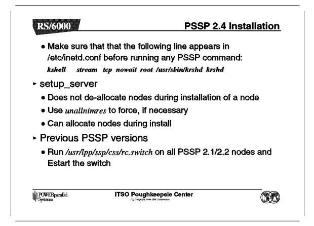
Checking the */etc/inetd.conf* entry is only required when running an AIX release of 4.3.1 or higher. Starting with AIX 4.3.1, SP software uses the AIX included security mechanism.
