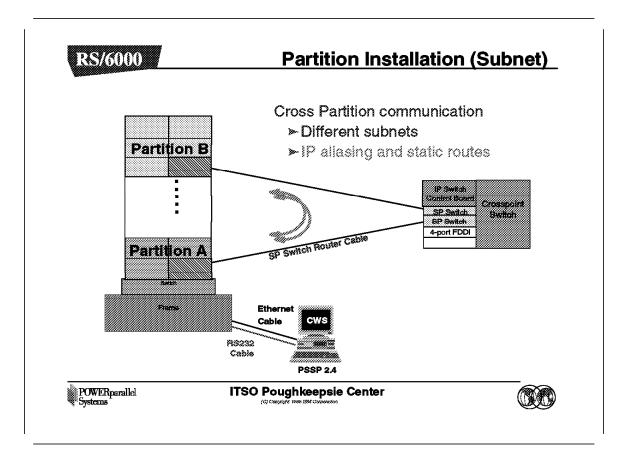
In this example, we install the RS/6000 SP such that SP Switch adapters in different partitions have different subnets. We assume the availability of a single frame RS/6000 SP system, with two partitions of eight nodes each. The IP address for the SP Switch network with a netmask of 255.255.255.0 is as follows:
