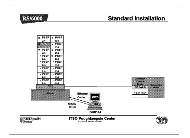
This example describes the steps for an installation of GRF into an RS/6000 SP system.
