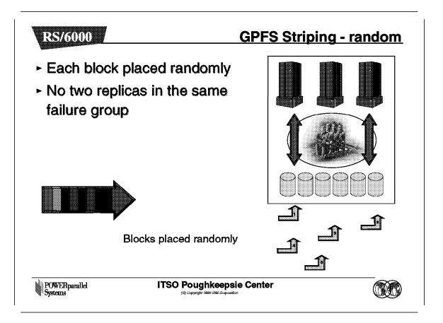
In the case of random striping, data blocks are placed randomly across the disks in the GPFS nodes. If failure groups are defined, the replicated data is stored in separate failure groups to cater for failures.
