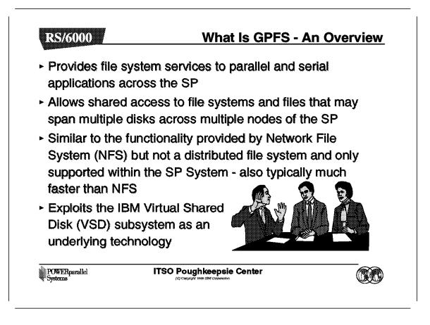
GPFS is a software product that is available on the SP. The software provides the functionality as shown, but it should be remembered that GPFS is only supported on the SP system. Systems external to the SP cannot run the GPFS software.
