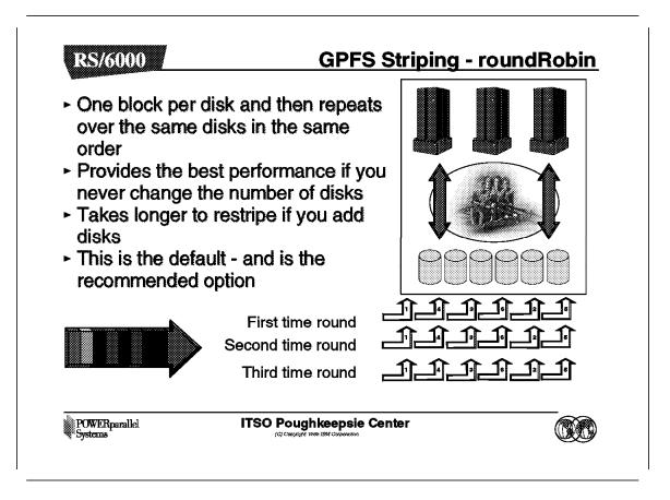
In the case of roundRobin striping, data is written in turn to each disk until all disks have received a block. Then another round of the disks begins, again writing a block each time, and accessing the disks in the same order.
