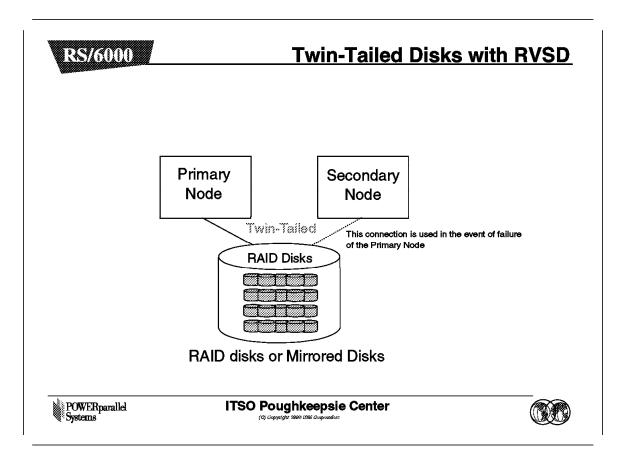
The recovery process shown here is the normal RVSD process working in conjunction with the high availability infrastructure.
