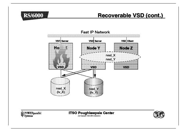
In this diagram, we see that Node X has failed. Node Y has taken ownership of the volume group that is twin-tailed and will vary on the volume group and make the VSDs available. In addition, RVSD will communicate with Group Services to inform other applications, such as Oracle, of the failure and recovery.
