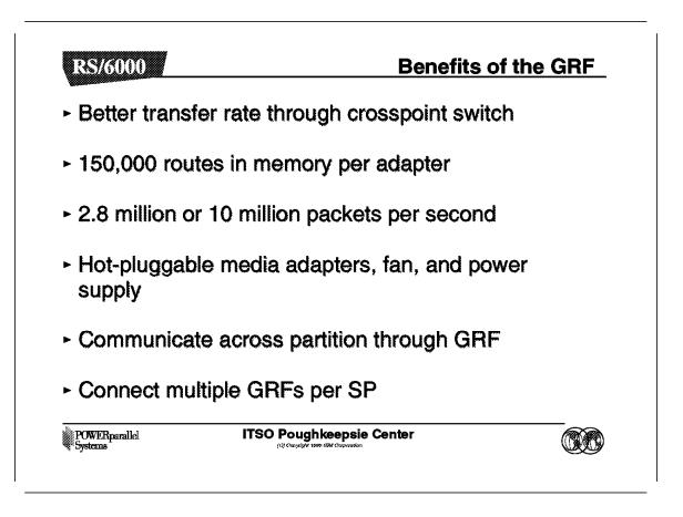
The crosspoint switch is a *non-blocking crossbar*. This architecture is faster than an RS/6000 SP node, in which media adapters communicate through a microchannel bus.
