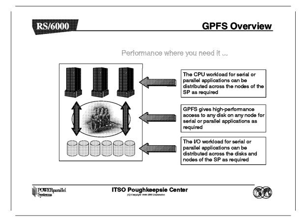
GPFS provides a truly parallel I/O solution for use within the SP. It can be exploited by both serial and parallel applications. It will allow for better balanced performance in many application environments, and will allow an application to exploit a number of nodes for I/O performance, as well as for CPU performance.
