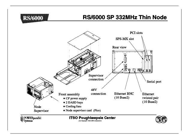
The CPU assembly includes the front assembly, which contains the power supply for the CPU assembly, two DASD bays, and the node supervisor card.
