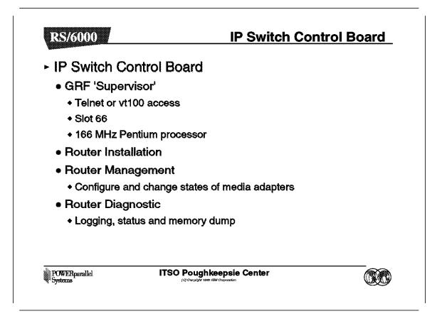
The control board, also known as the IP Switch Control Board, is accessed through Telnet or a locally attached VT100 terminal. The IP Switch Control Board is supplied with the GRF and is necessary for its operation. The VT100 terminal is not supplied with the GRF. It is only required for the installation of the GRF. After installation, all future access to the GRF is through Telnet to the IP Switch Control Board's administrative Ethernet.
