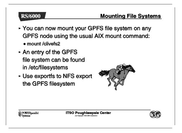
The GPFS file system, once created, can be mounted on any GPFS node in the normal way with the mount command.
