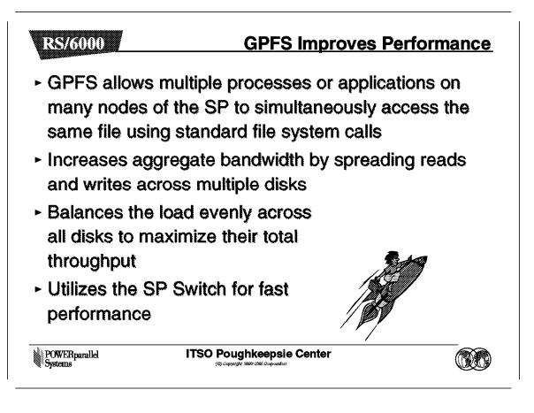
The GPFS software provides fast access across the SP Switch to disks attached to remote nodes within the SP. This results in extended flexibility and better performance.
