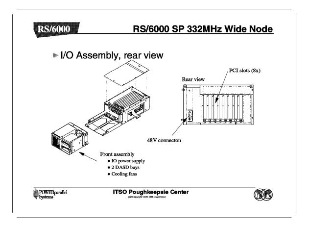
The I/O assembly includes the front assembly, which contains the power supply for the I/O assembly and two DASD bays.
