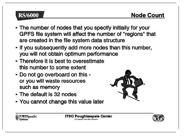
When determining how many nodes you will specify for your GPFS file system, it is important to remember that this value cannot be changed later.
