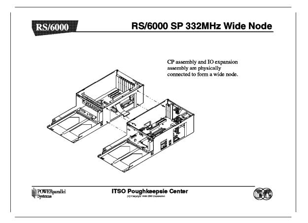
The CPU assembly and the I/O assembly are physically connected to form a wide node.
