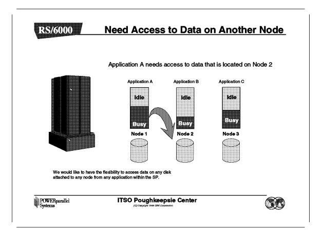
From a pure flexibility point of view, it is often very helpful to have access to data that resides on other nodes within the SP so that an application can run on any node within the SP, yet have access to data that it needs.
