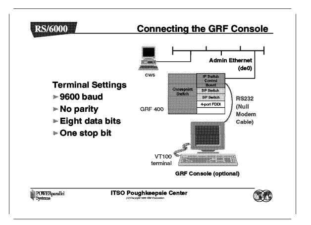
This figure shows how to connect the console to the GRF.
