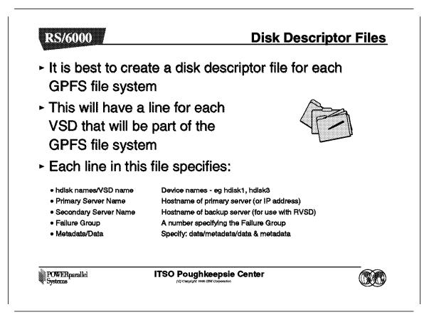
The information that you provide in a disk descriptor file is at the heart of a GPFS file system. It defines in detail exactly how the VSDs will be created. This information will be used by the create VSD commands.
