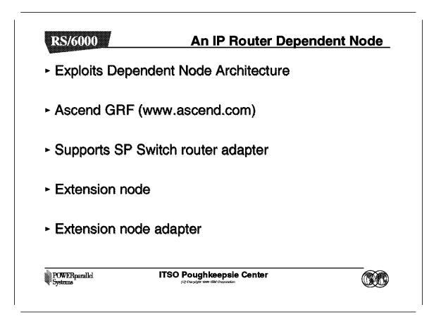
The first dependent node is actually a new SP Switch router adapter in a router. The purpose of this adapter is to allow the GRF, manufactured by Ascend, to forward SP Switch IP traffic to other networks. The GRF was known as the High Performance Gateway Node (HPGN) during the development of the adapter. IBM remarkets models of the GRF that connect to the SP Switch as the SP Switch router model 04S (9077-04S) and model 16S (9077-16S). These models are not available directly from Ascent.
