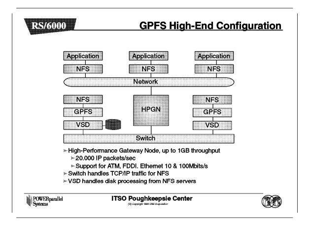
This configuration shows the use of the GRF node to allow NFS clients to access the GPFS file system with a high bandwidth.
