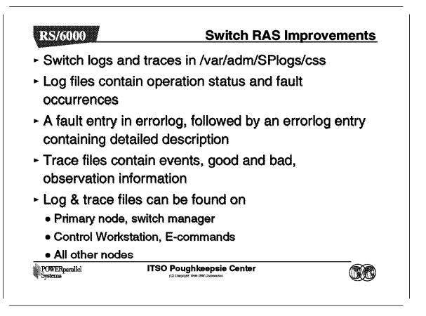
Better error logging and tracing facilities for the SP Switch are available with this new release of PSSP. Log and trace files are available on every node including the Control Workstation.
