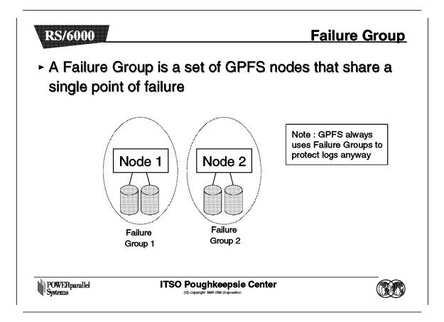
GPFS by default will assign a failure group at the node level for each disk in a GPFS file system.
