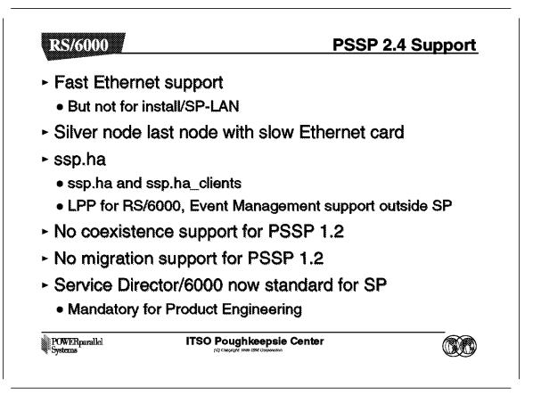
With PSSP 2.4, fast Ethernet adapters (100 BASE-T) are supported but not for the installation of the SP nodes.
