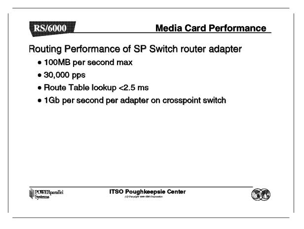
The SP Switch router adapter has the following performance characteristics:
