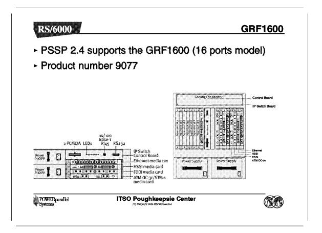
The first router node (GRF400) was announced in 1997. GRF1600 is a new model of the Switch Router which has among other characteristics, 16 slots for media cards. Refer to Chapter 6, "Dependent Node" on page 149 for more details about GRF1600.
