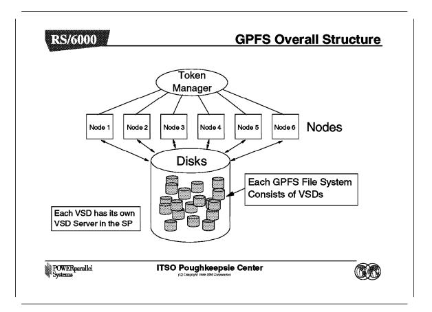
This diagram shows the overall structure of GPFS. Each GPFS file system is made up of a number of disks defined as VSDs. Each VSD can reside on any server node within the SP system. The file system writes data by striping across all of these VSDs.
