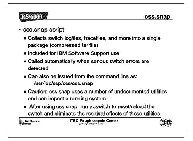
The css.snap script typically collects the following files: cable\_miswire, cable\_miswire.old, core (fault service daemon dump file), css.snap.log, css\_dump.out, daemon.stderr, daemon.stdout, dtbx.trace, dtbx.failed.trace, errpt.out (most recent errpt -a and errpt entries), flt, fs\_daemon\_print.file, netstat.out (current netstat -l css0 and netstat -m output), out.top, rc.switch.log, regs.out, router.log, scan\_out.log, scan\_save.log, tb\_dump.out, vdidl.out, and worm.trace.
