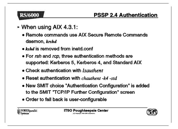
The remote commands (rcmds) include rsh, rcp, rlogin, telnet and ftp.
