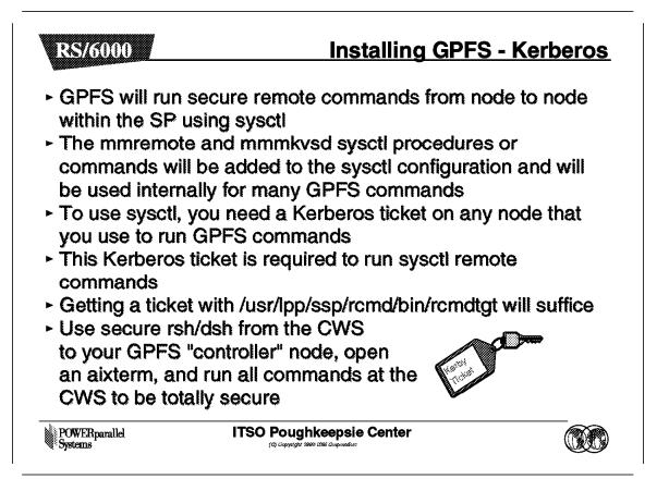
To use sysctl, you need a Kerberos ticket. Rather than type in a kinit command on the command line when working on a GPFS node, a remote ticket-granting ticket will be a better option.
