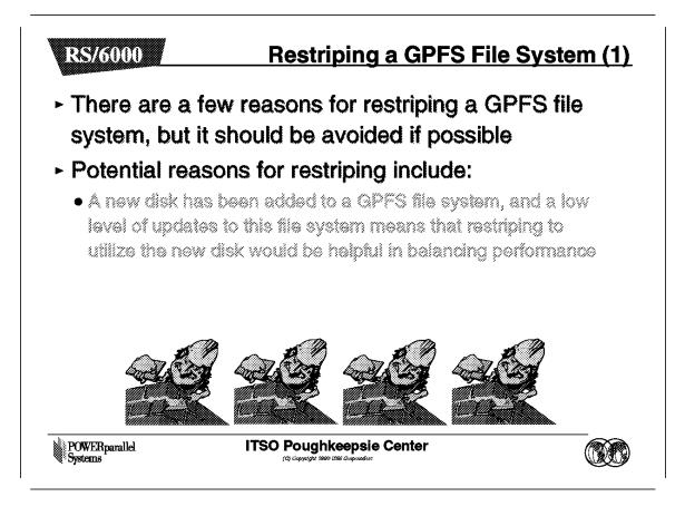
Restriping is an intensive process and should be avoided if possible.
