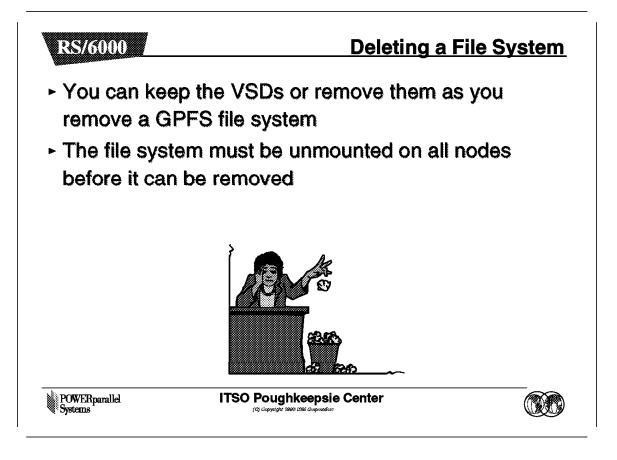
File systems can be removed when no longer required.
