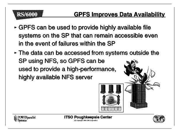
As we will see, GPFS uses the VSD technology to access remote disks. An extension for VSD is Recoverable Virtual Shared Disk (RVSD). This can provide disk takeover in the event of failure.
