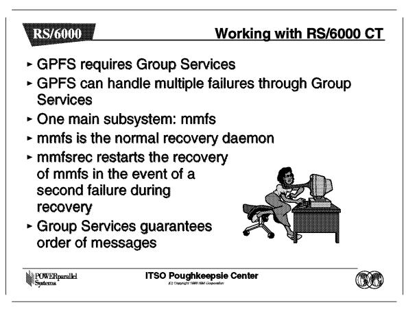
Both the mmfs and mmfsrec groups are registered with Group Services. The mmfs subsystem is the normal recovery mechanism. In the event of a second failure during the recovery, mmfsrec is used to ensure correct recovery.
