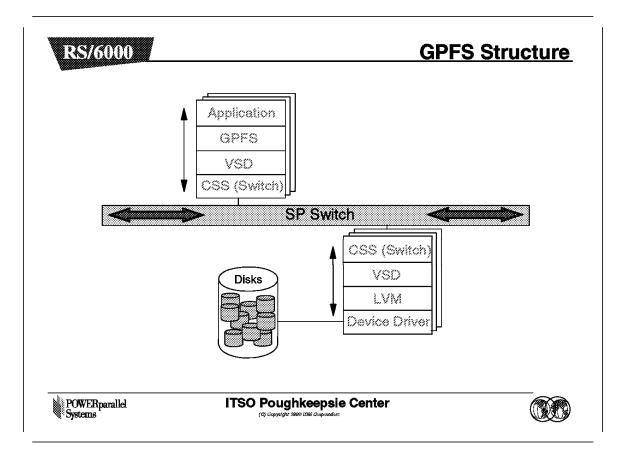
GPFS uses VSD to provide local or remote access to disks, as shown.
