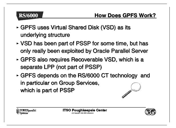
For access to remote disks, GPFS uses the tried and tested Virtual Shared Disk (VSD) that has been part of PSSP for a long time.
