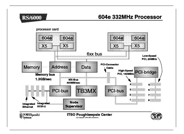
The RS/6000 SP 332MHz SMP nodes are functionally equivalent to an IBM RS/6000 7025-H50 workstation which uses a 6XX system bus, and a Peripheral Component Interconnect (PCI) bus architecture. TB3MX adapter is a variation on the TB3 adapter that plugs into the new Mezzanine (MX) bus.
