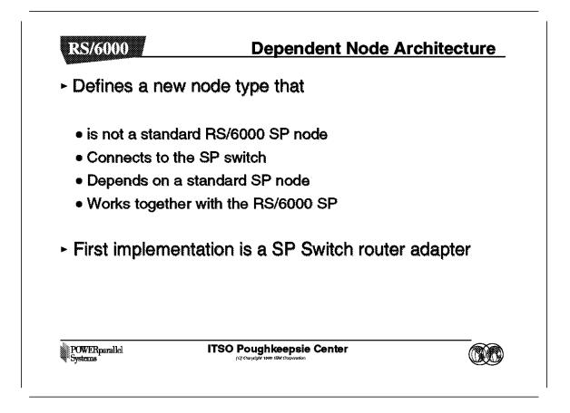
The Dependent Node Architecture refers to a processor or node, possibly not provided by IBM, for use with the RS/6000 SP.
