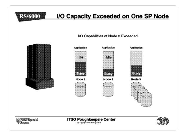
In this example, the capacity of node 3 has been exceeded from an I/O point of view. For example, adapter slots may have been filled and there is no room for more adapters to connect additional disks.
