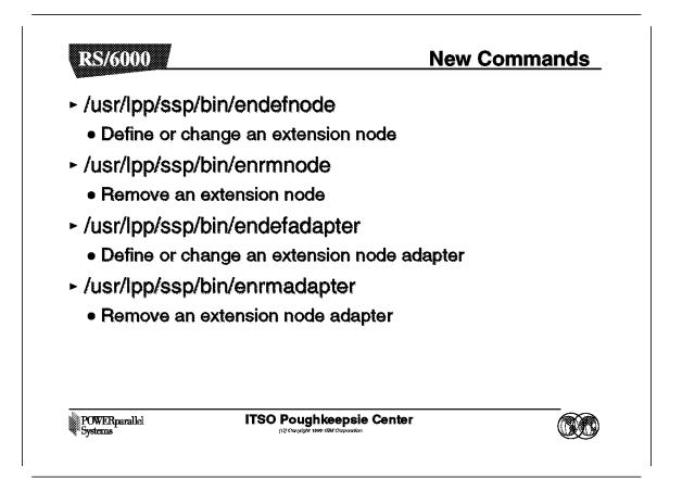
This figure shows four new commands that were added to manage the extension node. They have the same characteristics, which are as follows:
