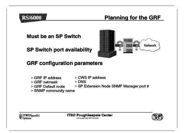
Before acquiring any model of the SP Switch Router, ensure that there are SP Switch ports available in the designated partition, and that the switch used in the RS/6000 SP is the 8-port or 16-port SP Switch.
