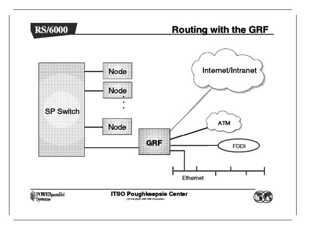
The GRF is a dedicated, high-performance router. Each SP Switch router adapter can route up to 30,000 packets per second and up to 100MB per second into the SP Switch network.
