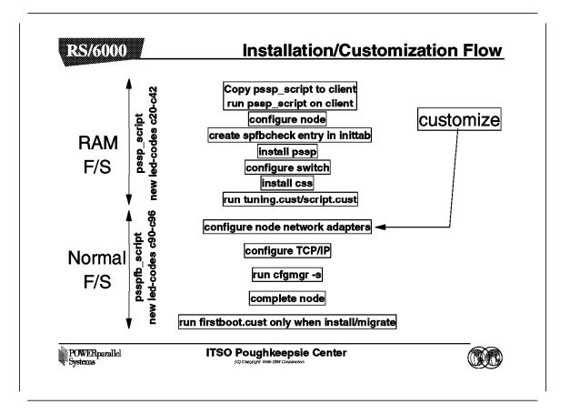
As previously noted, psspfb\_script is run during the first reboot of the node. It is run out of /etc/inittab after the /etc/firstboot script. It is invoked by a new module called spfbcheck, which functions in a manner similar to the base AIX module fbcheck, and which causes psspfb\_check to be run only after current reboot and then not again until reset by pssp\_script.
