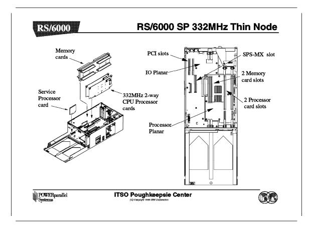
The SMP thin node is composed with CPU assembly only. It houses both the processor planar and I/O planar. The processor planar mounts the processor and memory, while the I/O planar mounts the SPS-MX slot and PCI slots.
