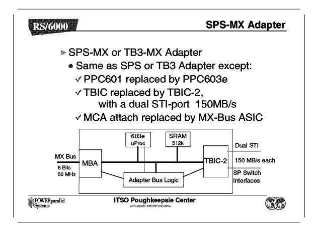
The TB3MX adapter is modeled after the TB3 adapter, but with the following changes:
