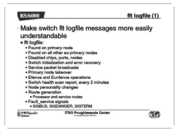
The flt log file was originally designed to log only "faults" in the switch fabric. However, it now contains a good deal of information for problem determination.
