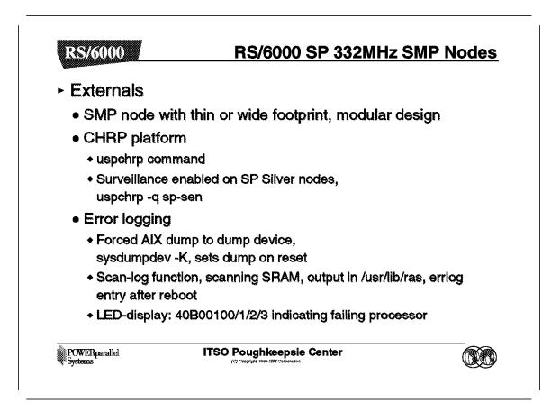
The RS/6000 SP 332MHz SMP nodes conform to the Common Hardware Reference Platform (CHRP), with some extensions due to the TB3MX adapter.
