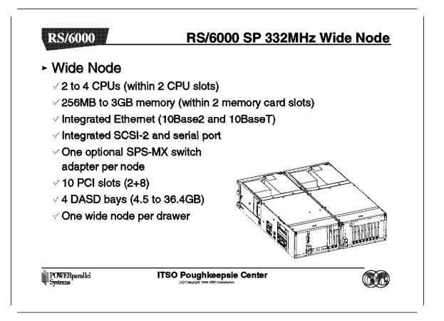
Wide nodes are now available in both a Symmetric Multiprocessing (SMP) configuration and in the previous uniprocessor configuration. All the RS/6000 SP 332MHz SMP wide nodes have Peripheral Component Interconnect (PCI) bus architecture.
