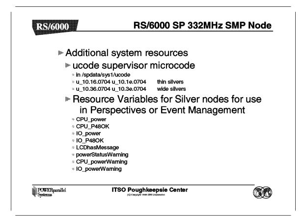
Supervisor microcode for the RS/6000 SP 332MHz SMP nodes is available in the /spdata/sys1/ucode directory. The files  $u_{10.16.0704}$  and  $u_{10.1e.0704}$  are for thin nodes, while  $u_{10.36.0704}$  and  $u_{10.3e.0704}$  are for wide nodes.
