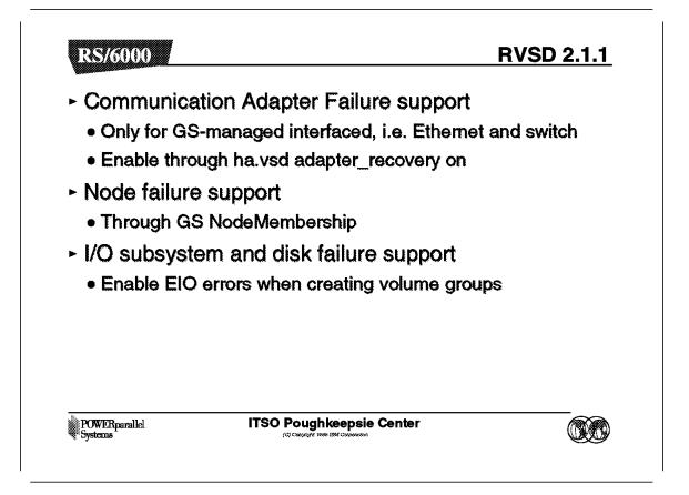
This new modification level of the IBM Recoverable Virtual Shared Disk provides a higher level of availability for the IBM Virtual Shared Disk subsystem by providing automatic recovery in the case of communication adapter failure. Should there be failure in the communication adapter, the IBM Recoverable Virtual Shared Disk will cause failover to the backup node. 1.3 General Parallel File System (GPFS)
