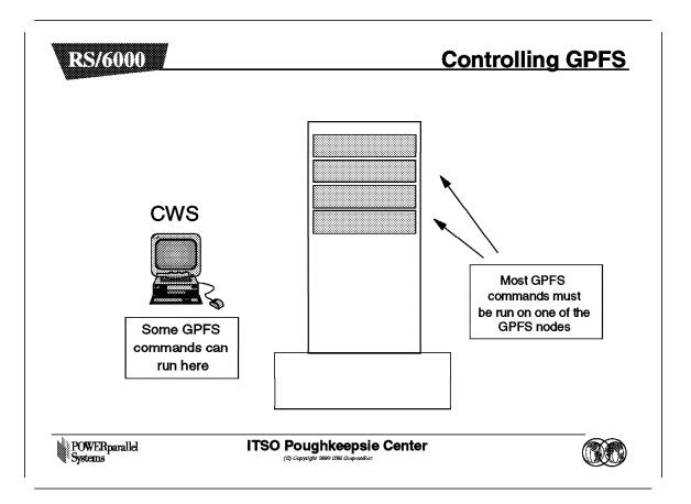
One of the things to note about GPFS is that much of the system management cannot be performed directly at the CWS. You need to be on a GPFS node to execute most GPFS commands.
