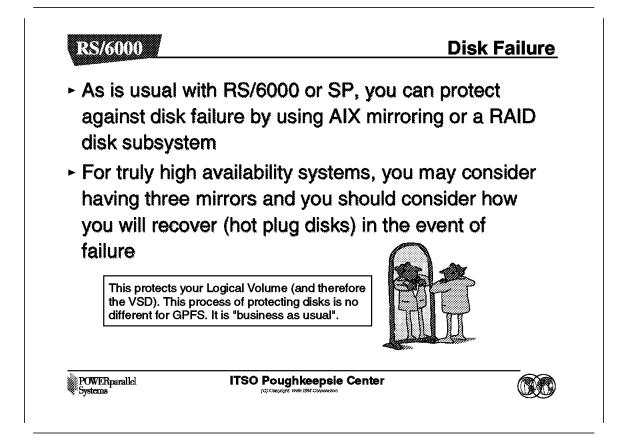
Disk mirroring or RAID disks should always be considered. The default solution would normally be SSA disks, with a loop attached to two nodes in the GPFS pool, and using AIX mirroring of the Logical Volume.
