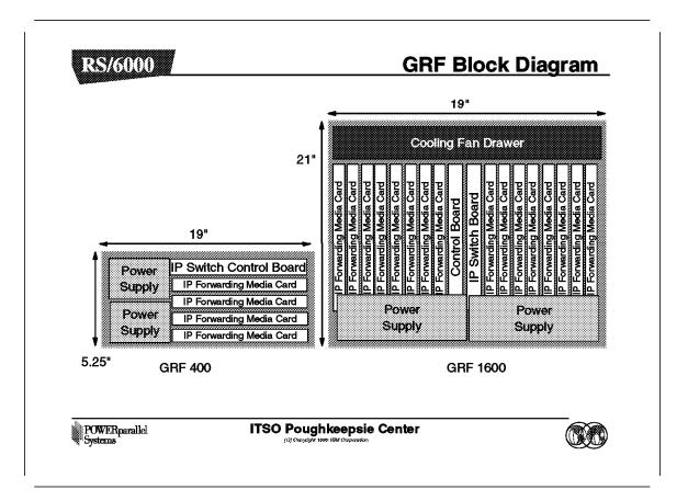
This figure shows the two GRF models: the 4-slot and the 16-slot model. Detailed descriptions of each follow.
