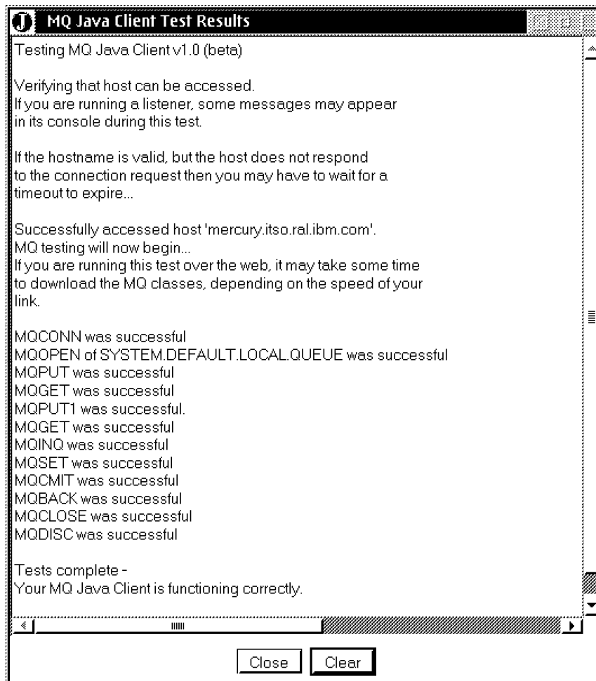
Figure 42. Verify Installation Results
