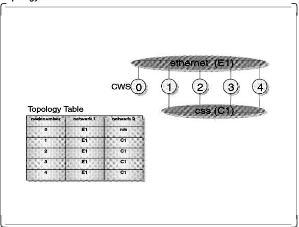
This diagram illustrates an example of Topology Services with the currently supported adapter networks in an RS/6000 SP environment. It consists of an Ethernet adapter network connecting all the nodes including the Control Workstation, and a switch network (CSS) which only connects the nodes, excluding the Control Workstation.
