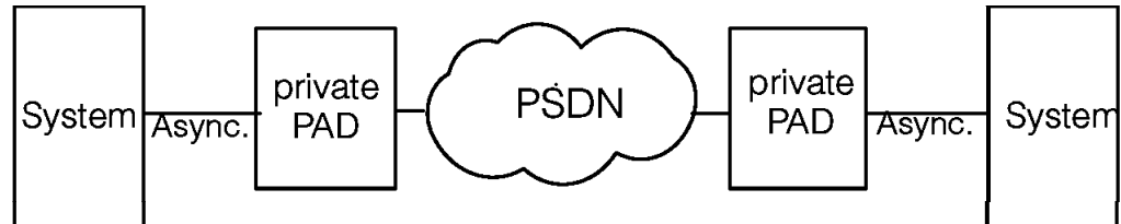
Figure 31. Private PADs Used to Carry Asynchronous Connections over a PSDN
