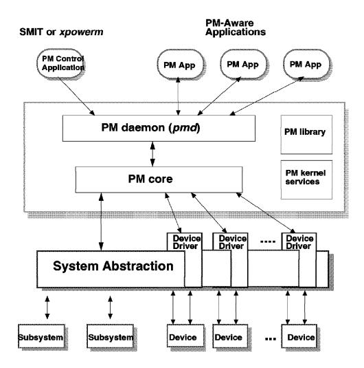
Figure 76. AIX Version 4.1.3 Power Management Components
