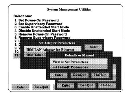
Figure 52. Adapter Parameters Submenu
