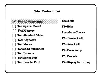
Figure 82. System Management Services - Device Test Menu
