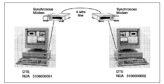
Figure 73. Two RISC System/6000s Connected Back-to-Back
