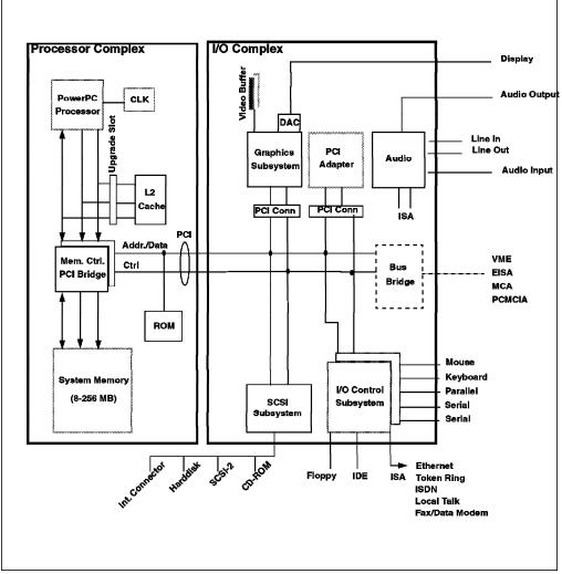
Figure 12. PowerPC Reference Platform Technical Workstation
