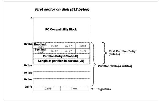
Figure 32. Boot Record Structure on RSPC Systems
