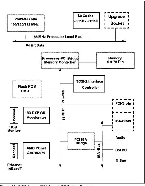
Figure 25. RISC System/6000 Model 43P System Diagram
