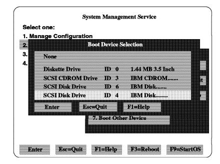
Figure 40. Boot Device Selection Submenu
