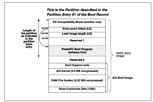
Figure 35. Structure of the RSPC Boot Image
