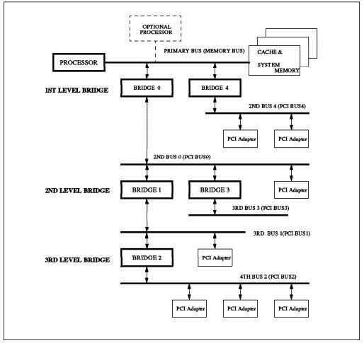
Figure 18. Multiple PCI Buses
