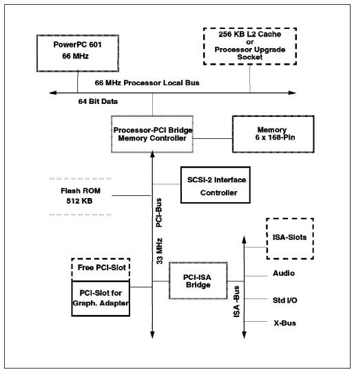
Figure 23. RISC System/6000 Model 40P System Diagram
