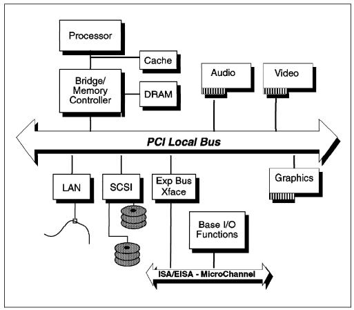
Figure 16. PCI System Block Diagram
