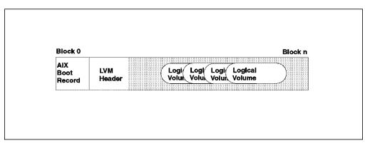
Figure 29. Hardfile Layout on a "Classical" RISC System/6000
