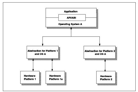
Figure 6. Architecture-Machine Abstractions
