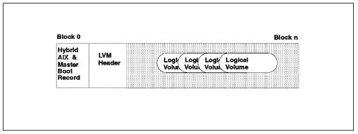
Figure 31. AIX Hardfile Layout on RSPC Systems
