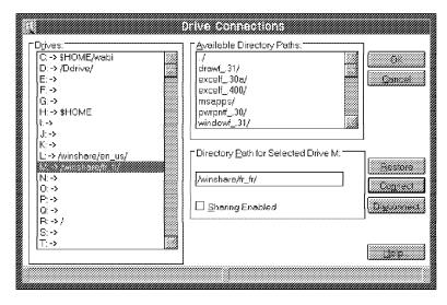
Figure 33. Example Filesystem Organization for Multiple NLS Applications. This picture shows the links between the AIX directories and the Windows drives (M: drive for French applications and L: drive for English applications).
