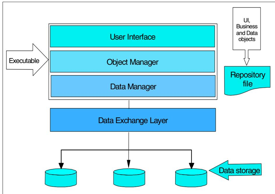
Figure 1. Siebel multi-layer architecture
