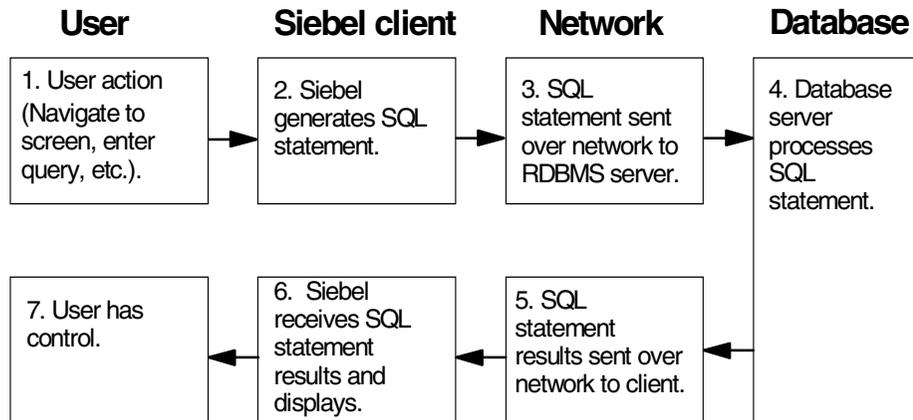
Figure 51. Components that contribute to user response time
