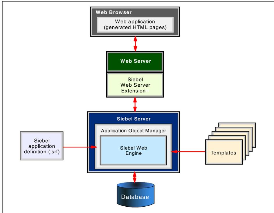
Figure 3. Main components for HTML Thin Clients
