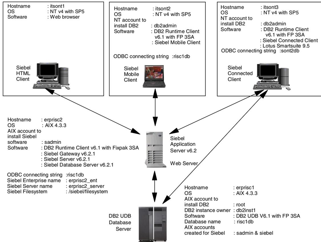
Figure 34. Environment of our DB2 and Siebel installation
