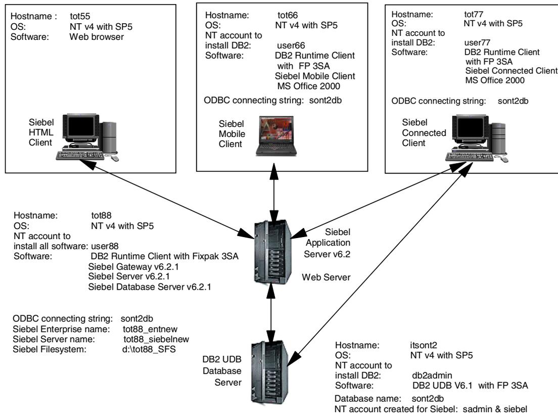
Figure 4. Environment of our DB2 and Siebel installation
