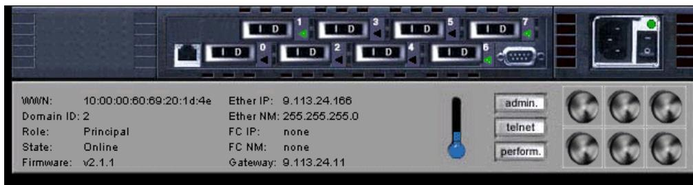
Figure 121. IBM 2109-S08 Fibre Channel switch
