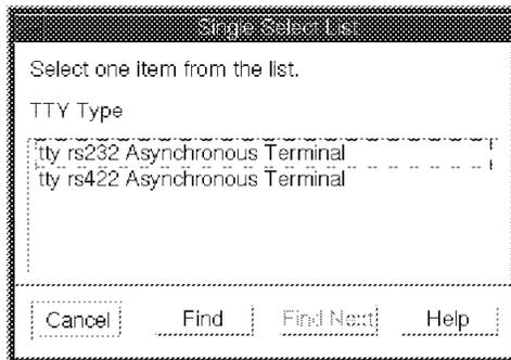
Figure 149. Single Select List Window for TTY Terminal Type Selection
