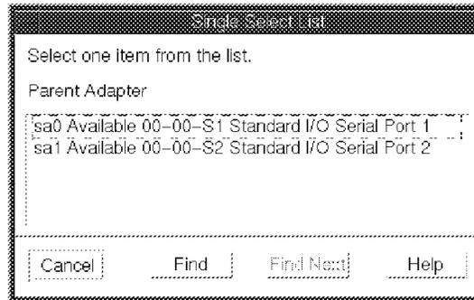
Figure 150. Single Select List Window for TTY Serial Port Selection
