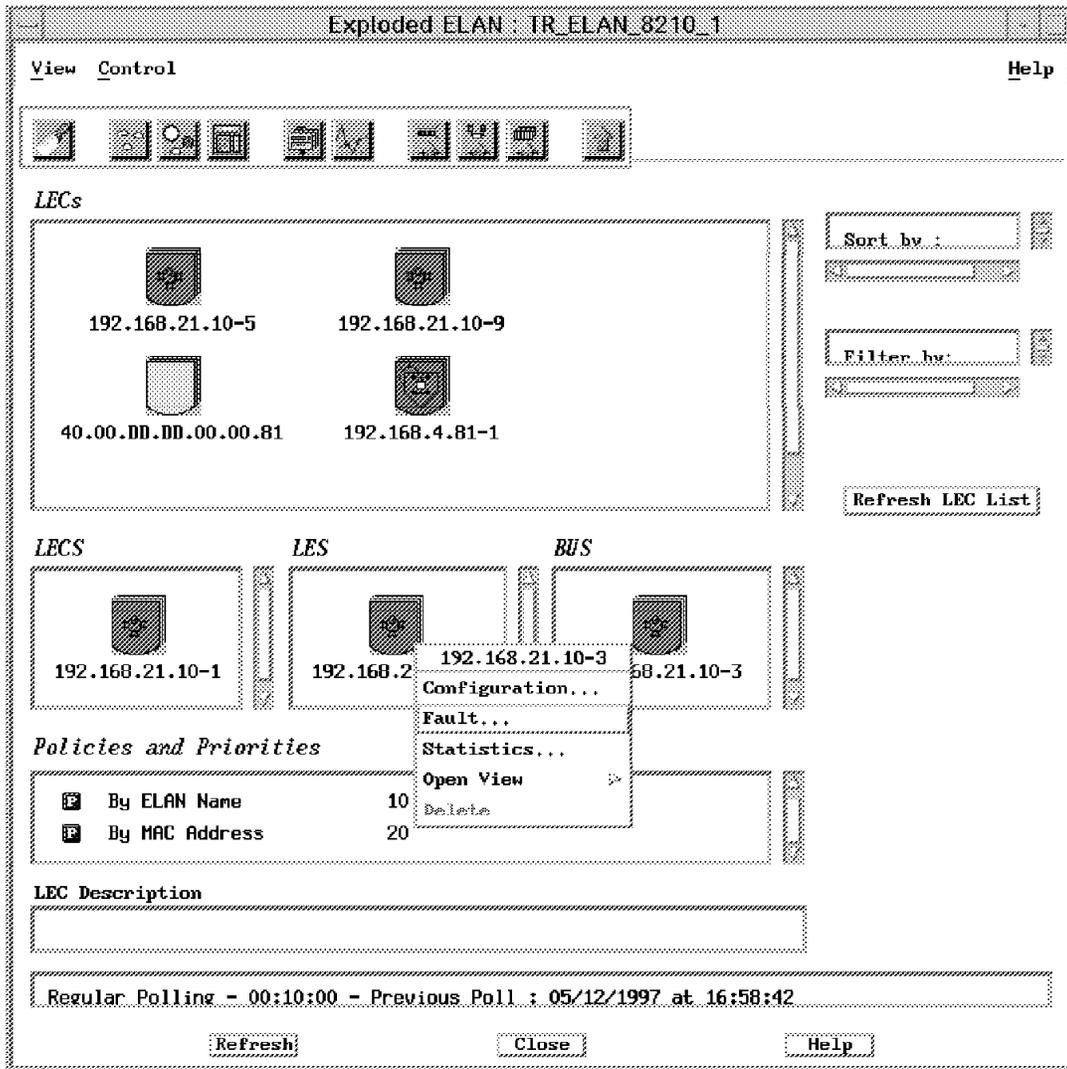
Figure 142. The LES Fault Management Panel
