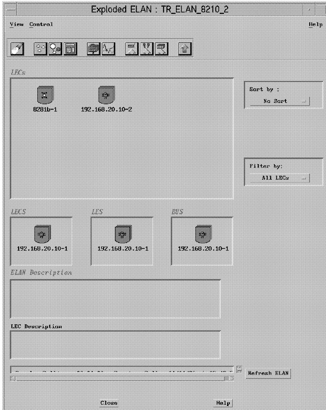
Figure 84. ELAN Topology Submap in First MSS after Cable Is Removed
