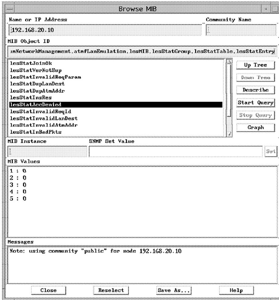
Figure 103. MIB Identifier for lesStatAccDenied
