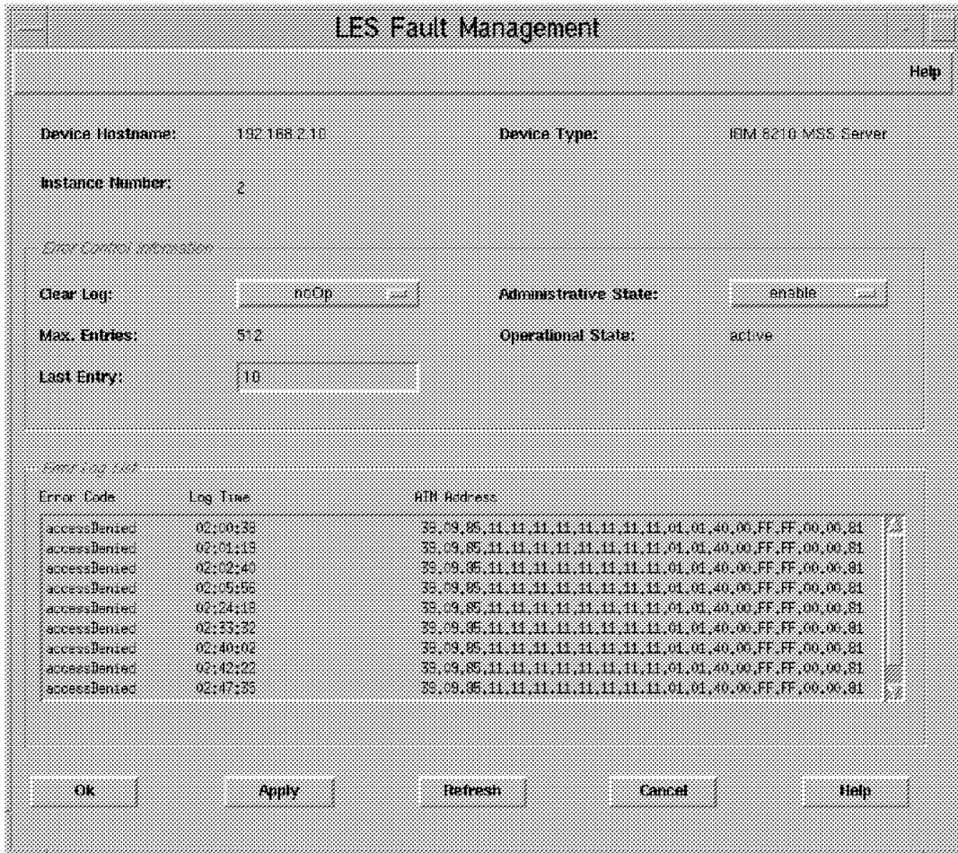
Figure 143. Errors Logged by the LES
