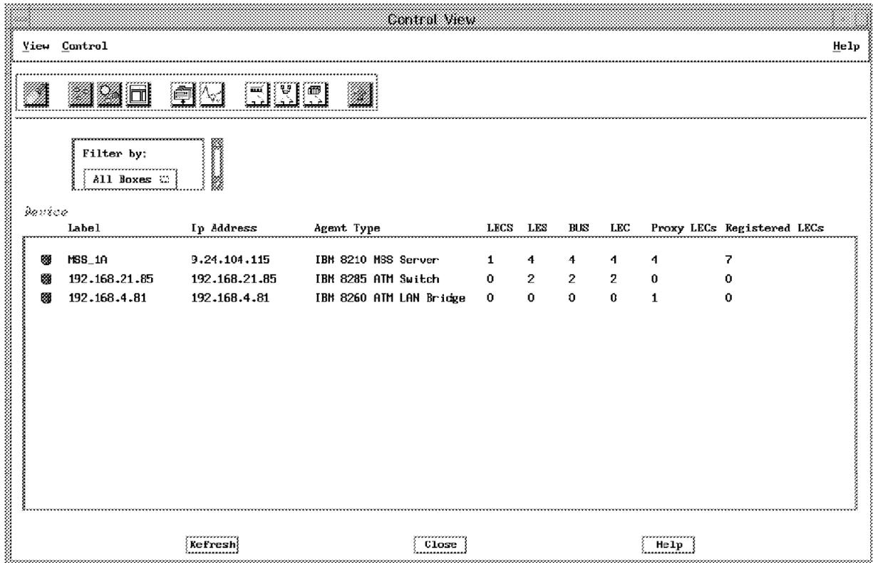
Figure 40. The Control View Panel
