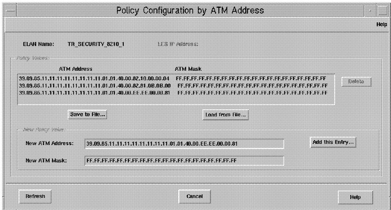
Figure 94. Adding the Manual LECs ATM Addresses to the Policy Value Table
