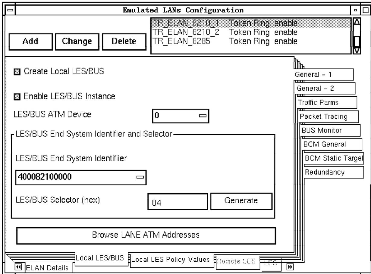
Figure 10. Emulated LAN Configuration
