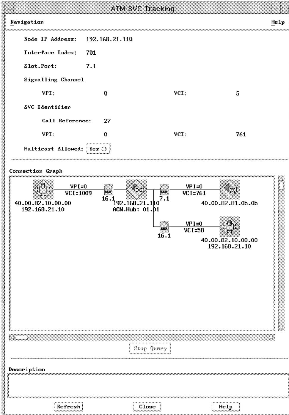
Figure 31. Tracking of a Multipoint SVC
