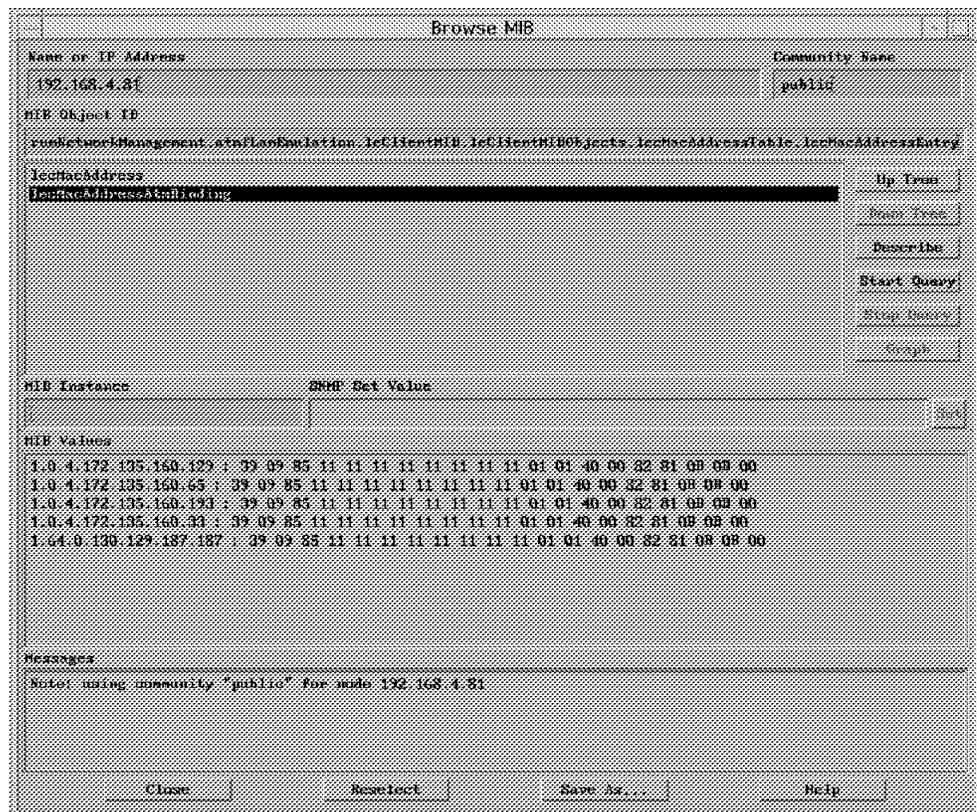
Figure 155. The Local Unicast MAC Addresses of an IBM 8281 ATM Bridge
