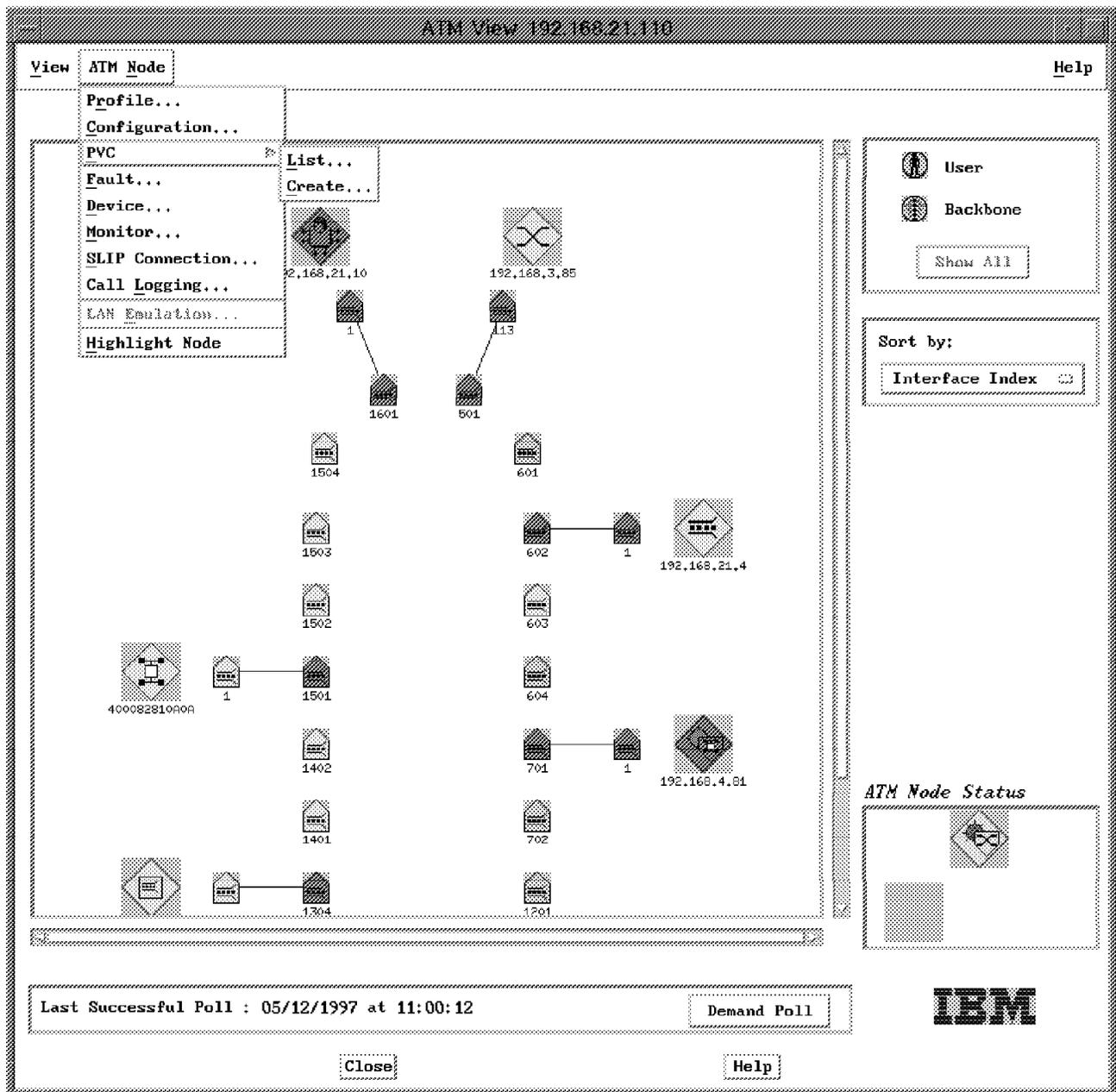
Figure 21. ATM View with ATM Node Menu
