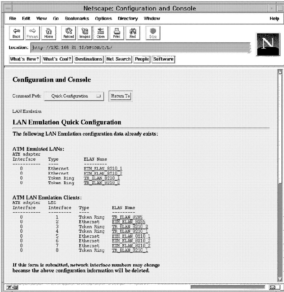
Figure 12. Quick Configuration for the IBM 8210
