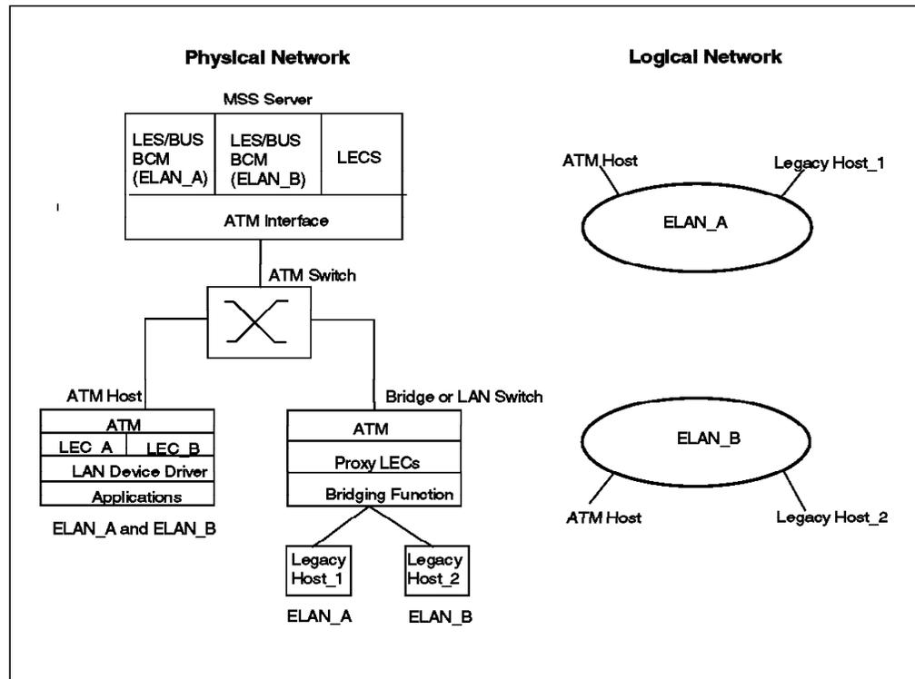
Figure 149. Physical and Logical Views of a Simple LAN Emulation Network
