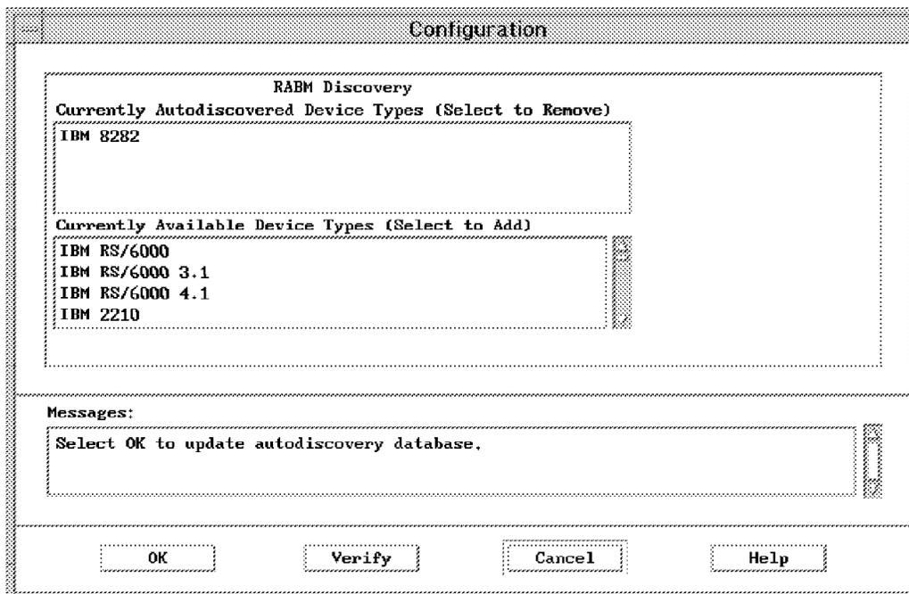
Figure 108. Router and Bridge Manager Modify RABM Auto-Discovery Settings
