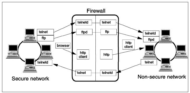
Figure 13. Firewall with Proxy Servers
