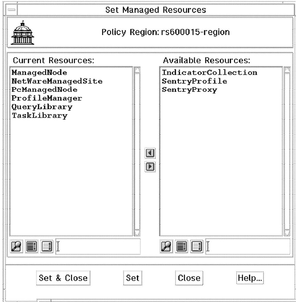
Figure 30. Assign Distributed Monitoring Resources As Managed Resources
