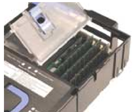
Memory mirroring provides greater reliability using industry-standard DIMMs.
