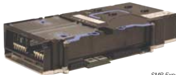
SMP Expansion Module takes a 4-way x440 to an 8-way x440.
