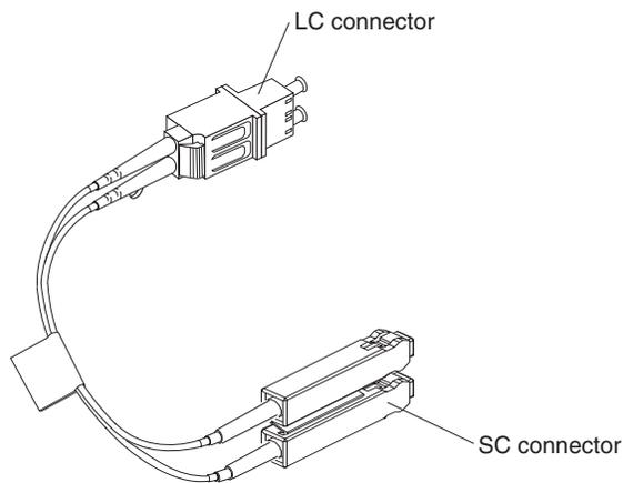
Figure 23. LC-SC Fibre Channel cable adapter
