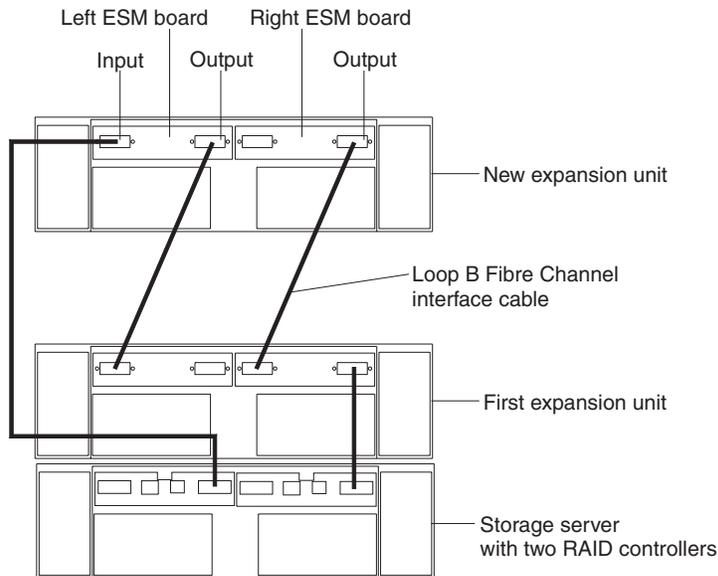
Figure 35. FAST EXP700 redundant loop configuration
