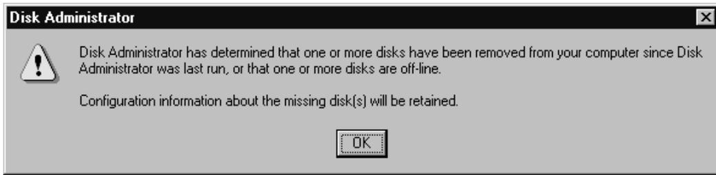
3. Because disks were balanced across the two RAID controllers before the error occurred, every other disk shows in the Disk Administrator as off-line, and the partition information section is grayed out, showing the following:
