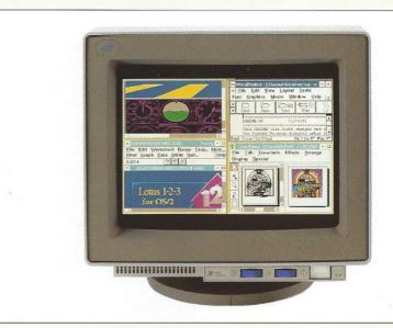
Perfectly matched to Personal System/2® computers, the 9515's footprint makes it right for almost any desktop. And it's extremely convenient and easy to use thanks to its Tilt/Swivel stand, front-mounted on/off, brightness and contrast controls, and its comfortably sized viewing area. In addition, you can free up extra desk space with the optional Lift/Tilt/Swivel stand.
