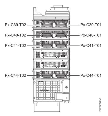
Figure 41. I/O hub card locations (lower nodes)
