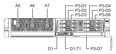
Figure 17. Front view of base model with six small-form factor (SFF) bays
