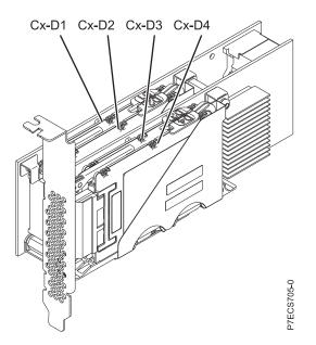
Figure 16. PCIe SAS RAID and SSD adapter locations
