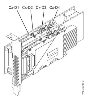
Figure 29. PCIe SAS RAID and SSD adapter locations
