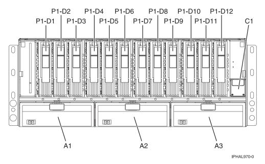
Figure 48. I/O enclosure (drawer model, front) or (stand-alone model on its side, front)
