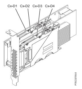
Figure 8. PCIe SAS RAID and SSD adapter locations
