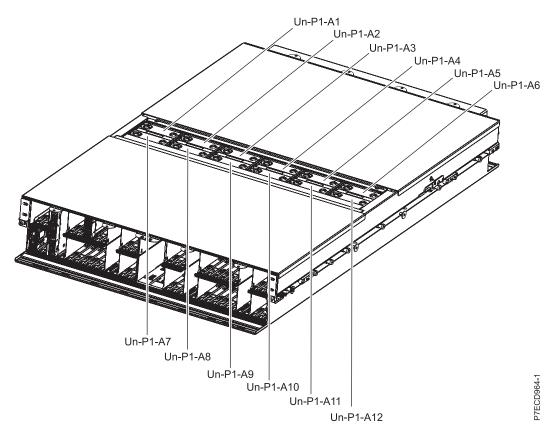
Figure 46. Bulk power fan (BPF) locations
