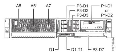
Figure 18. Front view of model with three SFF bays (optional)
