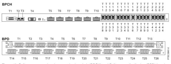
Figure 43. Bulk power control and communications hub (BPCH) and Bulk power distribution (BPD) locations
