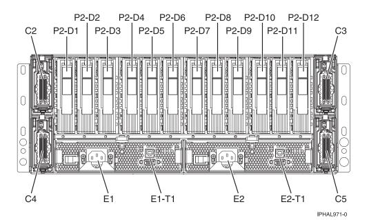
Figure 49. I/O enclosure (drawer model, back)
