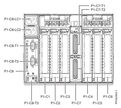
Figure 51. Rear view of unit.
