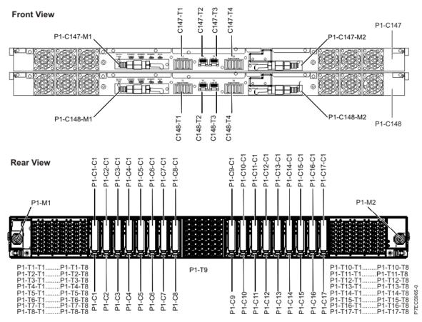
Figure 47. Distributed converter and control assembly (DCCA) and PCIe riser locations
