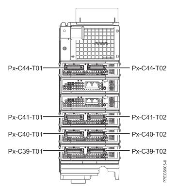
Figure 40. I/O hub card locations (upper nodes)
