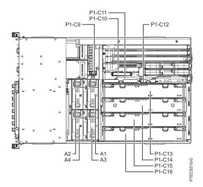
Figure 31. Rack top view
