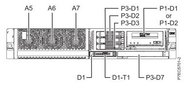
Figure 24. Front view of model with three SFF bays (optional)
