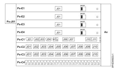
Figure 37. Bulk power assembly (BPA). Front is Un-P1 and back is Un-P2.
