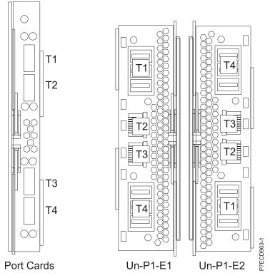
Figure 45. Bulk power assembly (BPA) connector locations
