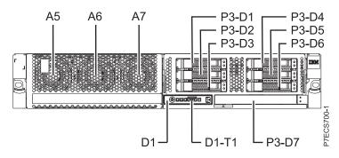
Figure 23. Front view of base model with six small-form factor (SFF) bays
