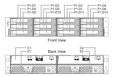
Figure 42. Disk drive locations for the 58/86 disk-drive enclosure
