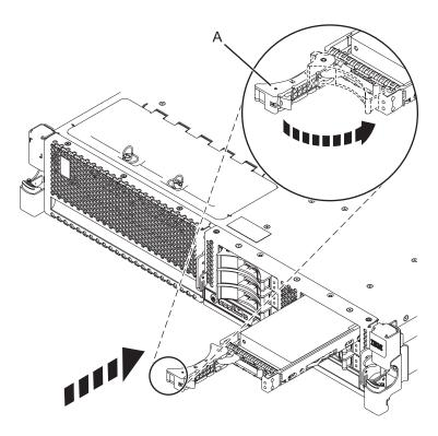
Figure 25. Installing a disk drive in the system
