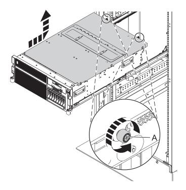
Figure 82. Removing the service access cover
