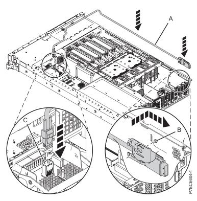
Figure 29. Replacing the SAS cable
