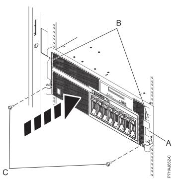
Figure 116. Replacing the thumbscrews
