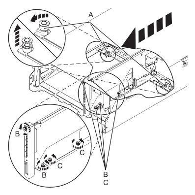
Figure 69. Removing the SAS conduit card and midplane
