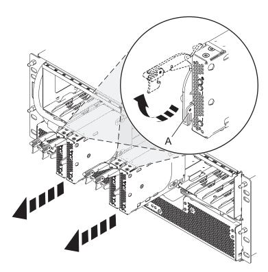
Figure 72. Removing the SAS expander card.
