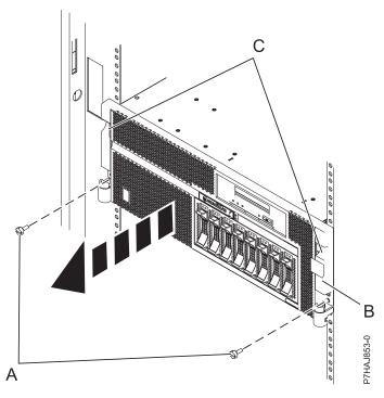
Figure 90. Removing the front cover
