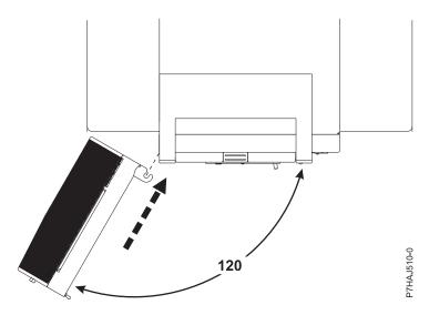
Figure 81. Installing the front door
