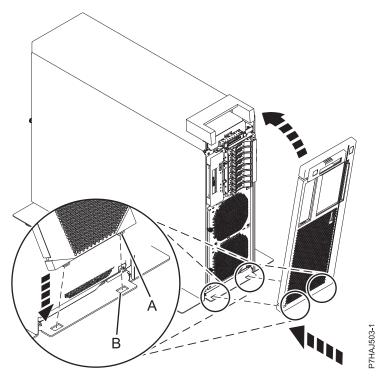
Figure 80. Installing the front cover
