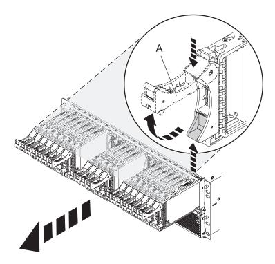
Figure 61. Removing the drives from the backplane
