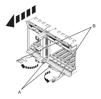
Figure 68. Removing the I/O system board
