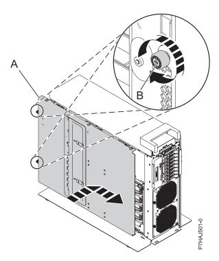
Figure 86. Installing the inside service access cover
