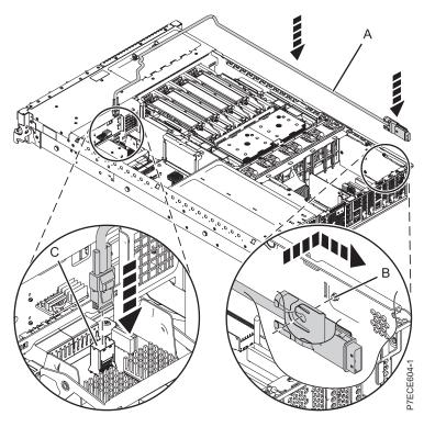
Figure 28. Installing the SAS cable
