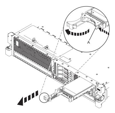
Figure 18. Removing a disk drive from the system
