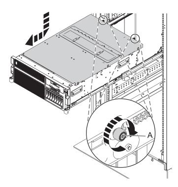
Figure 85. Installing the service access cover
