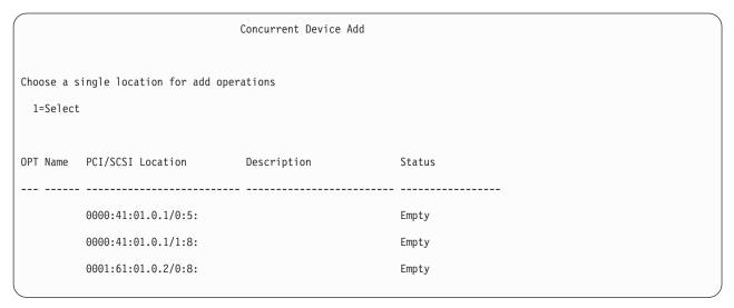
Figure 23. Example Concurrent Device Add display
