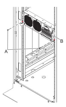
Figure 105. Placing the system in the service position
