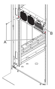
Figure 107. Placing the system into the operating position
