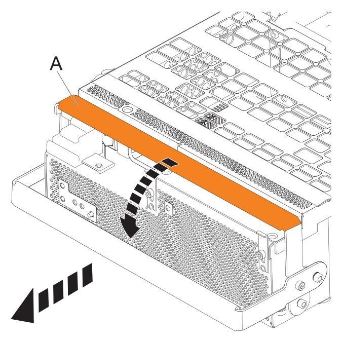
Figure 65. Remove the offline converter assemblies
