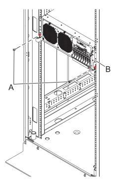
Figure 110. Placing the system into the operating position
