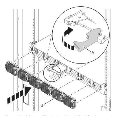
Figure 11. Installing a solid-state drive in the 58/88 PCle storage enclosure
