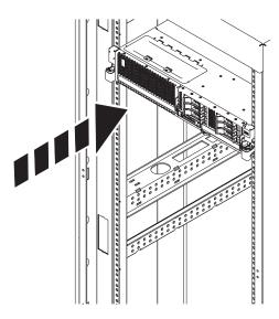
Figure 104. Placing the system into the operating position
