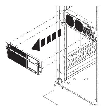
Figure 77. Removing the front cover
