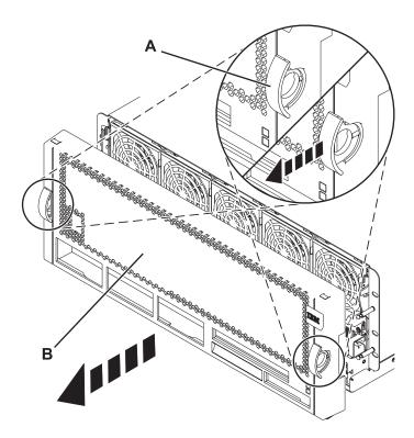
Figure 94. Removing the front cover
