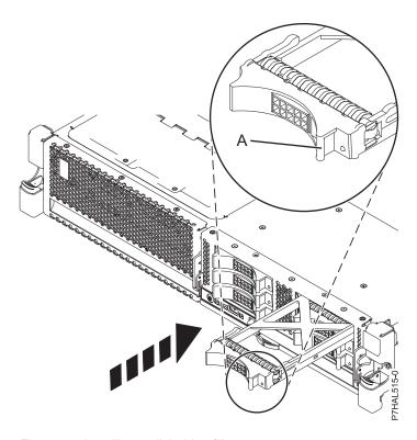
Figure 31. Installing a disk drive filler
