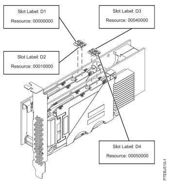
Figure 32. PCIe RAID and SSD SAS adapter locations
