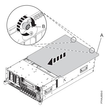
Figure 93. Installing the service access cover
