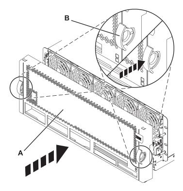
Figure 101. Installing the front cover
