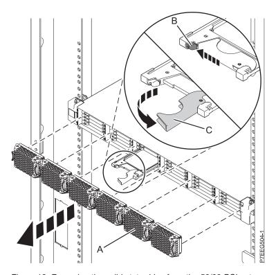
Figure 13. Removing the solid-state drive from the 58/88 PCle storage enclosure
