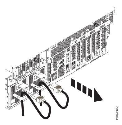
Figure 117. Removing the power cords for a rack-mounted system
