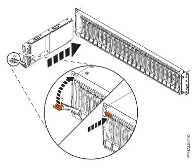
Figure 7. Installing the disk drive in the 58/87 disk drive enclosure
