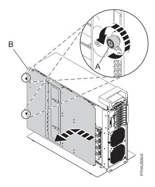
Figure 84. Removing the inside service access cover
