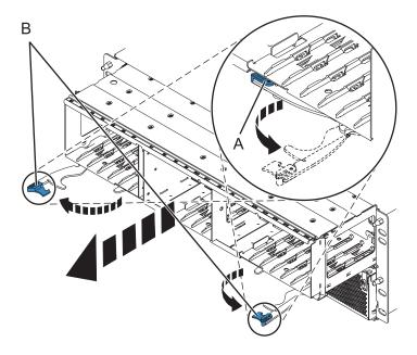
Figure 63. Removing the backplane from the enclosure
