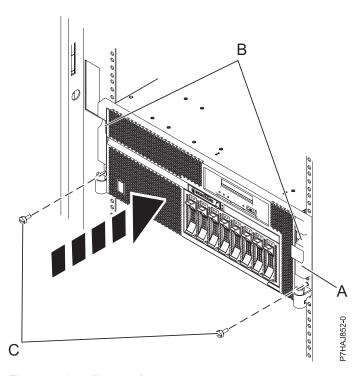
Figure 91. Installing the front cover
