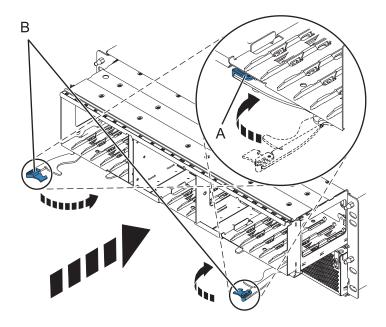
Figure 60. Installing the backplane on a rack-mounted model
