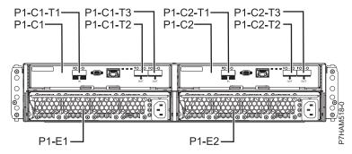
Figure 45. Rear view of the 58/87 disk drive enclosure
