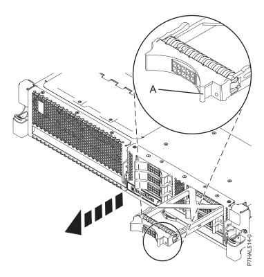
Figure 30. Removing a disk drive filler
