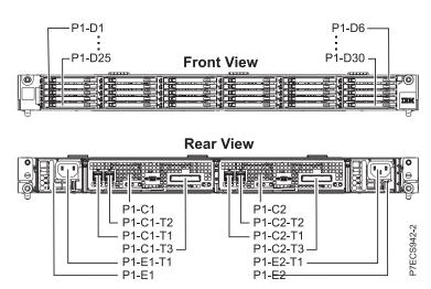
Figure 47. Front and rear views of the 58/88 PCIe storage enclosure showing the solid-state drive locations
