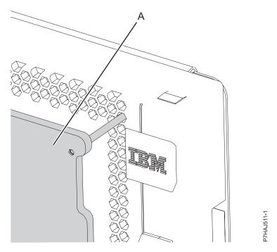
Figure 96. Aligning the cover removal tool
