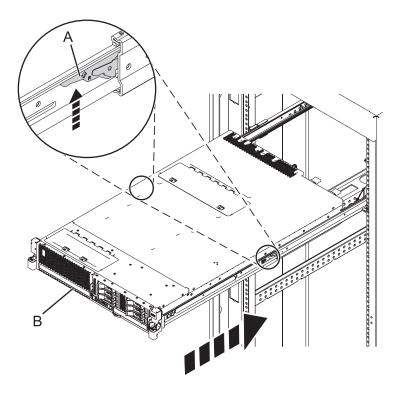
Figure 103. Unlocking the safety rail latches
