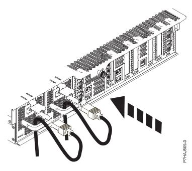
Figure 121. Connecting the power cords
