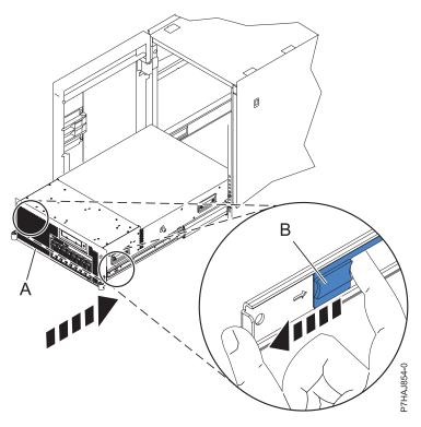
Figure 115. Releasing the rail safety latches
