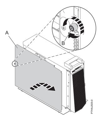
Figure 87. Installing the outside service access cover
