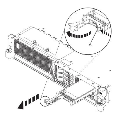
Figure 19. Removing a disk drive from the system
