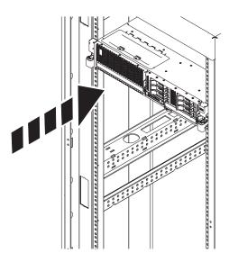
Figure 113. Placing the system into the operating position
