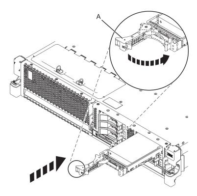
Figure 1. Installing the disk drive in the system
