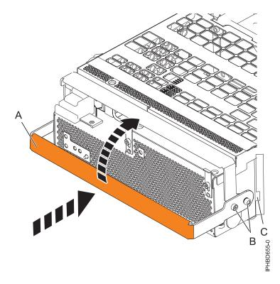
Figure 59. Replacing a power supply
