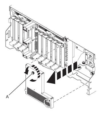
Figure 67. Removing the power cord plate
