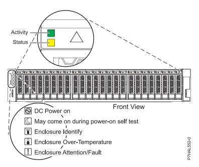
Figure 46. Front view of the 58/87 disk drive enclosure showing the service indicators
