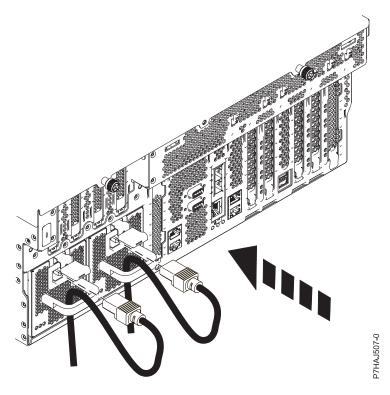
Figure 119. Connecting the power cords
