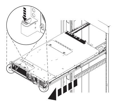
Figure 102. Placing the system in the service position
