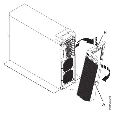
Figure 78. Removing the front cover
