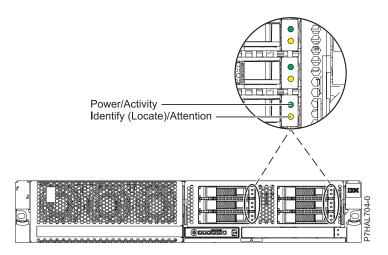
Figure 35. Service indicators locations for systems with six SFF bays
