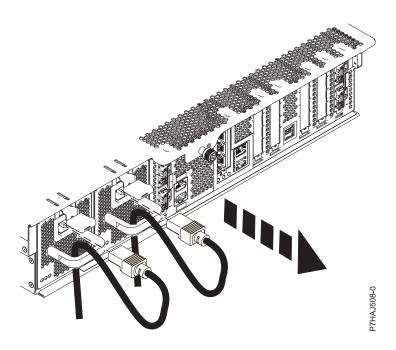
Figure 120. Removing the power cords
