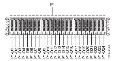
Figure 44. Front view of the 58/87 disk drive enclosure showing the disk-drive locations
