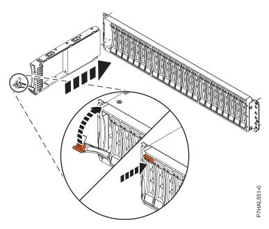
Figure 2. Installing the disk drive in the 58/87 disk drive enclosure
