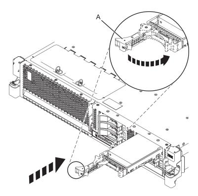
Figure 9. Installing the drive in the system
