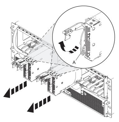
Figure 62. Removing the port card from the backplane
