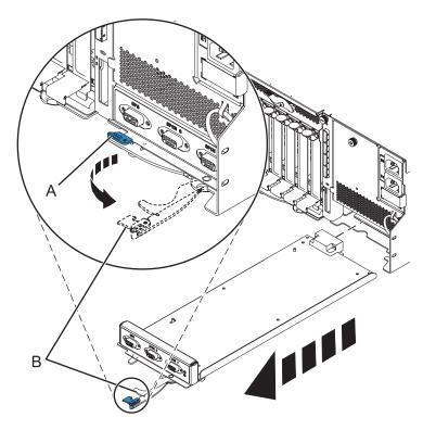
Figure 66. Remove the enclosure management controller
