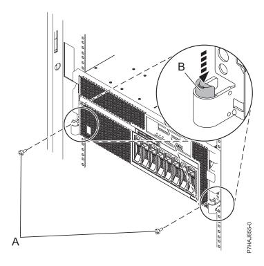
Figure 114. Releasing the rack latches
