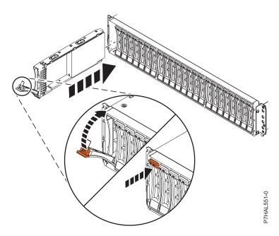
Figure 10. Installing the disk drive in the 58/87 disk drive enclosure
