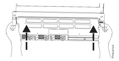
Figure 97. Cover removal tool use
