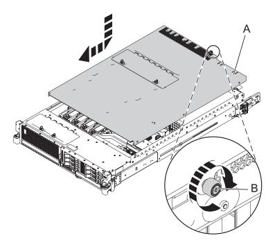
Figure 89. Installing the service access cover
