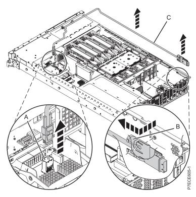
Figure 27. Removing the external SAS port
