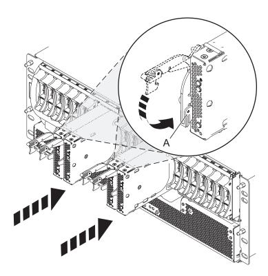
Figure 71. Installing the SAS expander card
