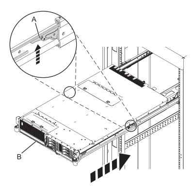
Figure 112. Unlocking the safety rail latches
