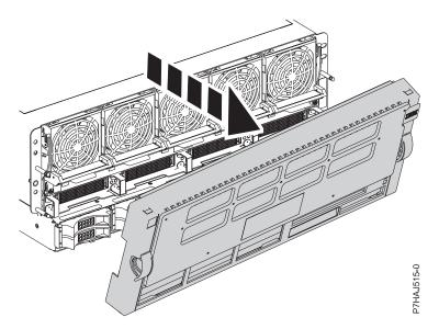
Figure 100. Removing the cover
