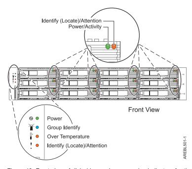
Figure 43. Front view of disk drive enclosure service indicators for the 58/86
