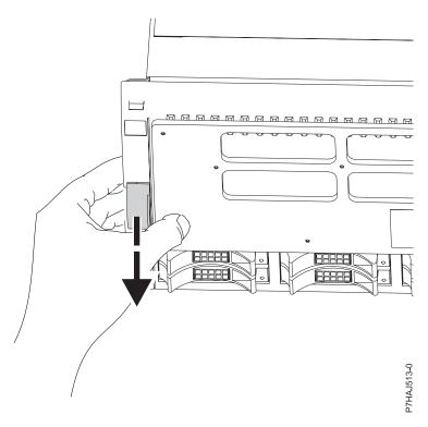
Figure 98. Releasing the cover latches
