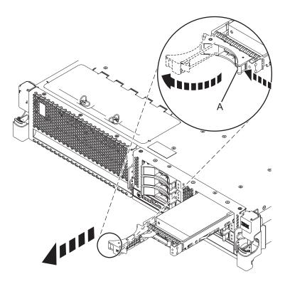
Figure 12. Removing a disk drive from the system
