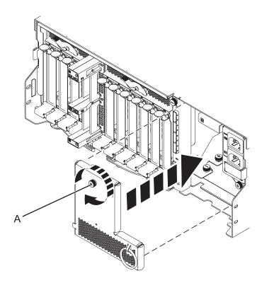
Figure 56. Installing the power cord plate
