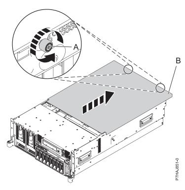
Figure 92. Removing the service access cover
