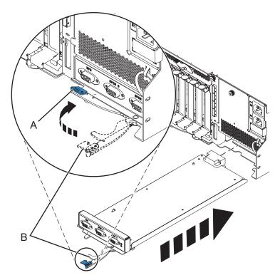
Figure 57. Replacing the enclosure management controller
