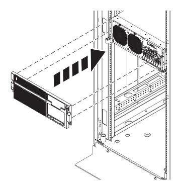
Figure 79. Removing the front cover
