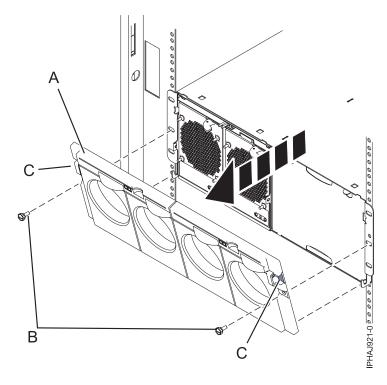
Figure 75. Remove the front cover for model 14G/30
