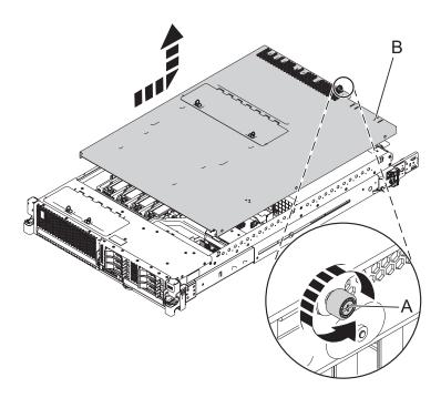
Figure 88. Removing the service access cover
