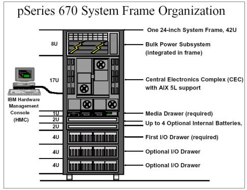
Figure 2-23 7040-671 internal structure
