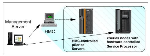
Figure 4-8 Hardware control capability in CSM
