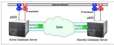
Figure 5-2 A basic two-server HACMP cluster configuration
