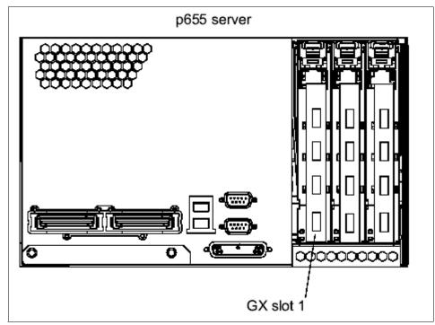
Figure 2-33 p655 SNI GX bus slot location
