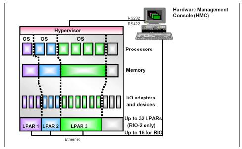
Figure 2-3 LPAR concept diagram
