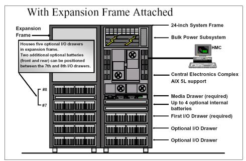
Figure 2-27 7040-681 pSeries 690 internal structure
