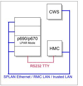
Figure 3-11 Cluster 1600 with one HMC, one pSeries and CWS
