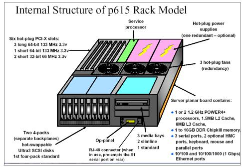
Figure 2-9 7029-6C3 internal structure
