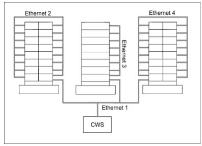
Figure 3-3 CWS with one Ethernet card; one node has two adapters
