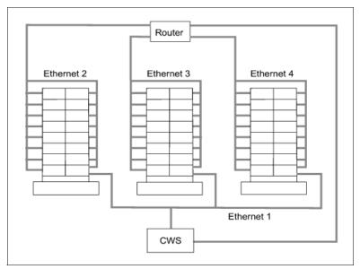
Figure 3-4 Ethernet topology for multi-frame system
