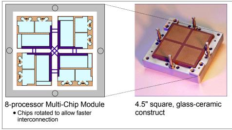
Figure 2-5 POWER4 Multi-Chip Module (MCM)
