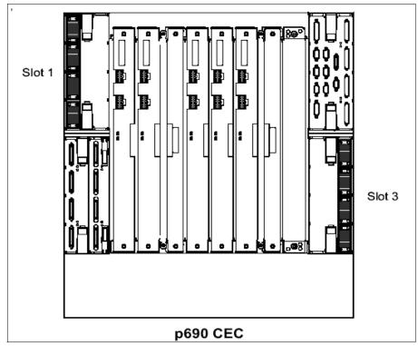
Figure 2-32 p690 SNI GX bus slots location
