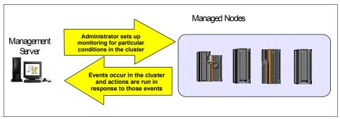
Figure 4-10 Event monitoring and automated response in a CSM cluster
