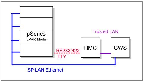
Figure 3-5 The RMC LAN uses the SP LAN and the trusted network
