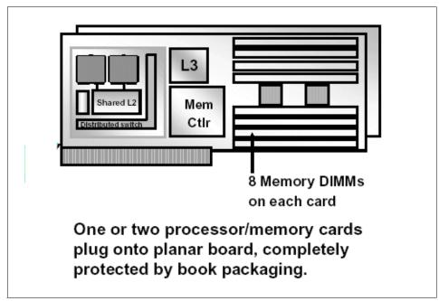
Figure 2-7 POWER4+ processor card layout
