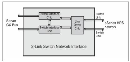
Figure 3-16 Conceptual view of a 2-Link SNI card
