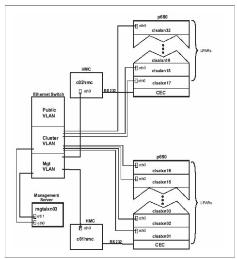
Figure 3-15 Conceptual diagram for series cluster
