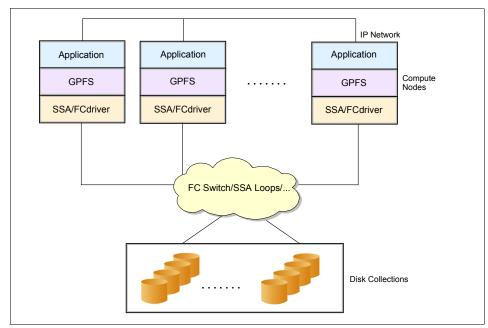
Figure 4-13 GPFS in a direct-attached SAN environment
