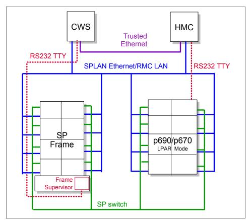
Figure 3-13 SP frame and pSeries with SP-Switched LPARs
