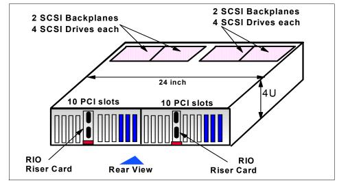
Figure 2-24 p670 I/O drawer rear view
