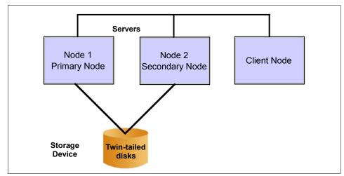
Figure 4-15 Simplified view of a twin-tailed disk
