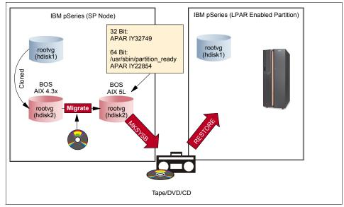
Figure 5-4 alt\_diskinstall process
