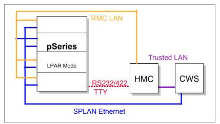
Figure 3-8 Each function has its own physical network
