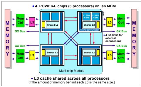
*Figure 2-6* Multi-Chip Module with L2, L3, and memory
