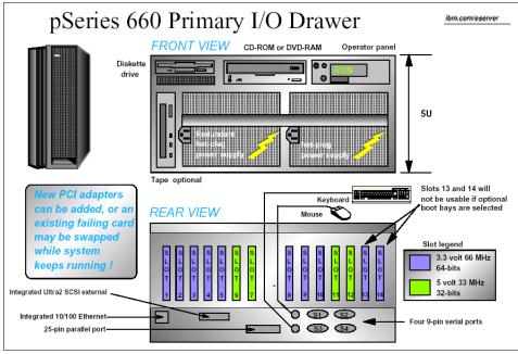
Figure 2-36 p660 IO drawer internal structure
