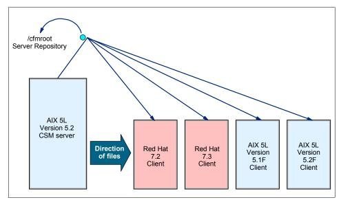
Figure 4-7 Configuration file maintenance and propagation using CFM
