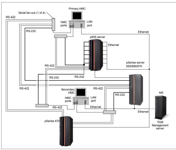
Figure 3-19 Redundant layout for pSeries in a Cluster 1600
