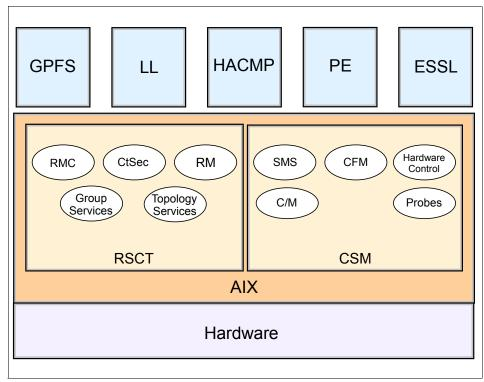
Figure 4-2 Functional diagram of Cluster 1600 software on CSM
