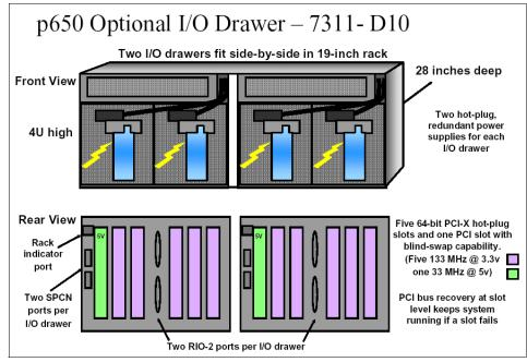
Figure 2-15 7311-D10 internal structure
