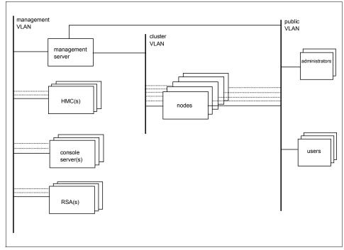
Figure 3-14 VLAN configuration
