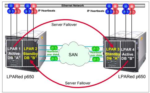
Figure 5-3 HACMP configuration in an LPAR environment
