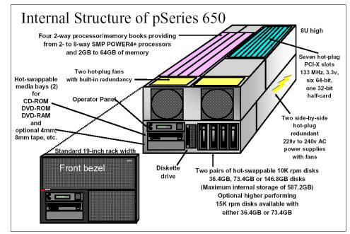
Figure 2-14 7038-6M2 internal structure
