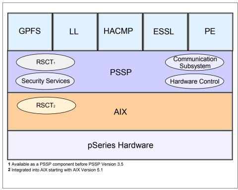
Figure 4-1 Functional diagram of Cluster 1600 software on PSSP
