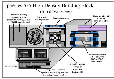
Figure 2-18 7039-651 internal structure
