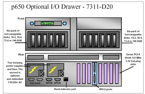
Figure 2-16 7311-D20 internal structure (p650)
