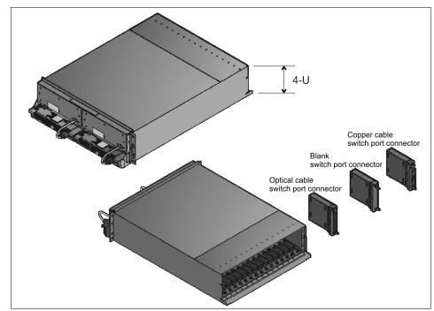
Figure 2-30 HPS switch internal structure
