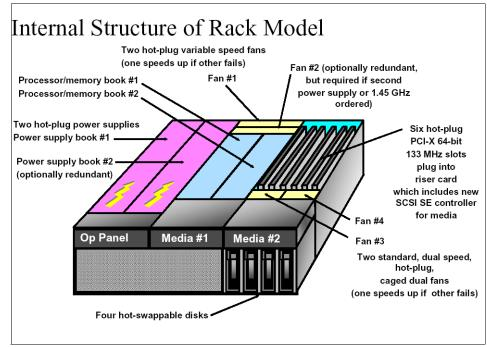
Figure 2-11 7028-6C4 internal structure
