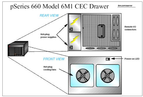
Figure 2-35 p660-6M1 internal structure
