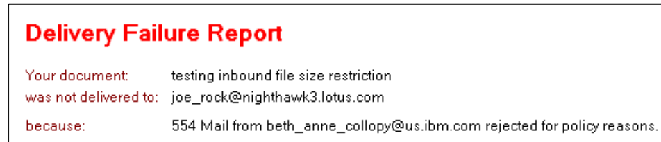
Figure 4-7 Delivery Failure Report with 554 SMTP response code
