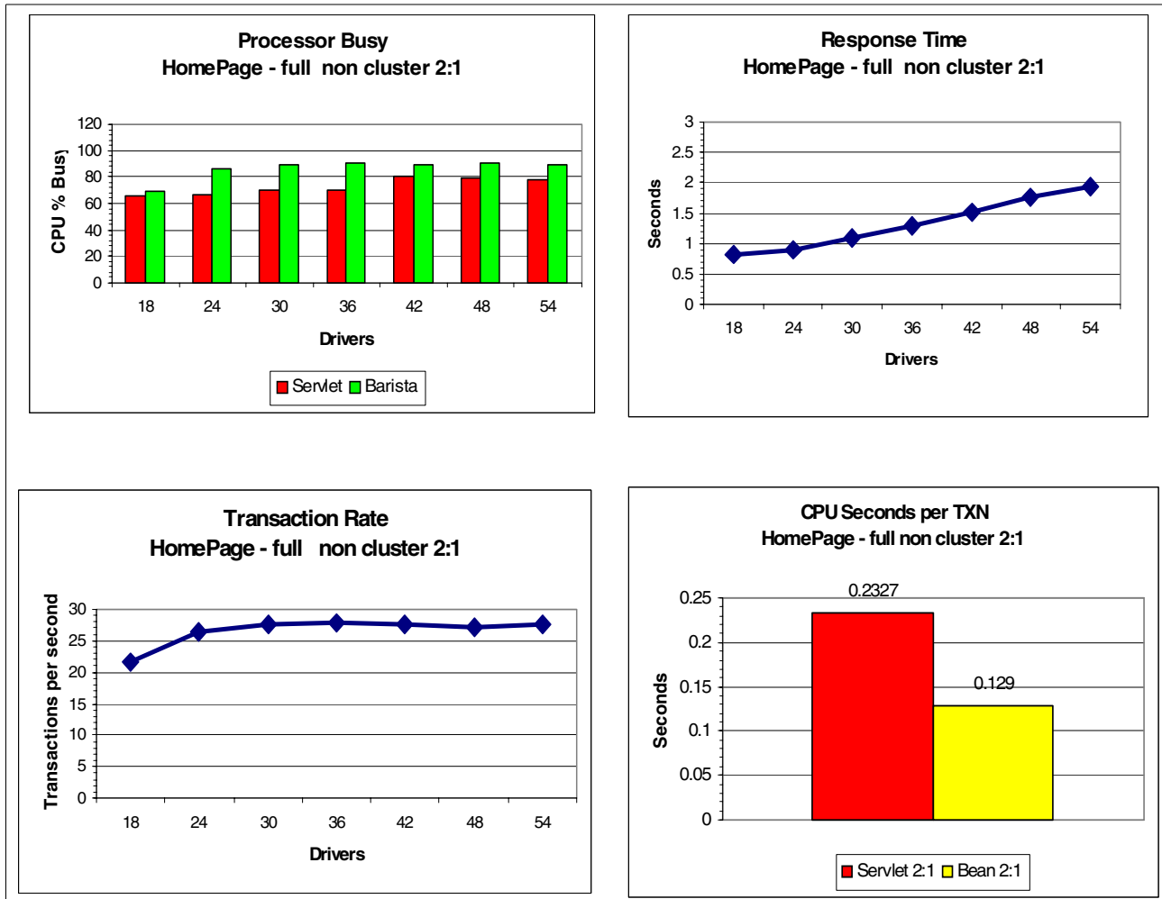
Figure 8-8 Results of Barista test (two presentation servers and one business logic server)
