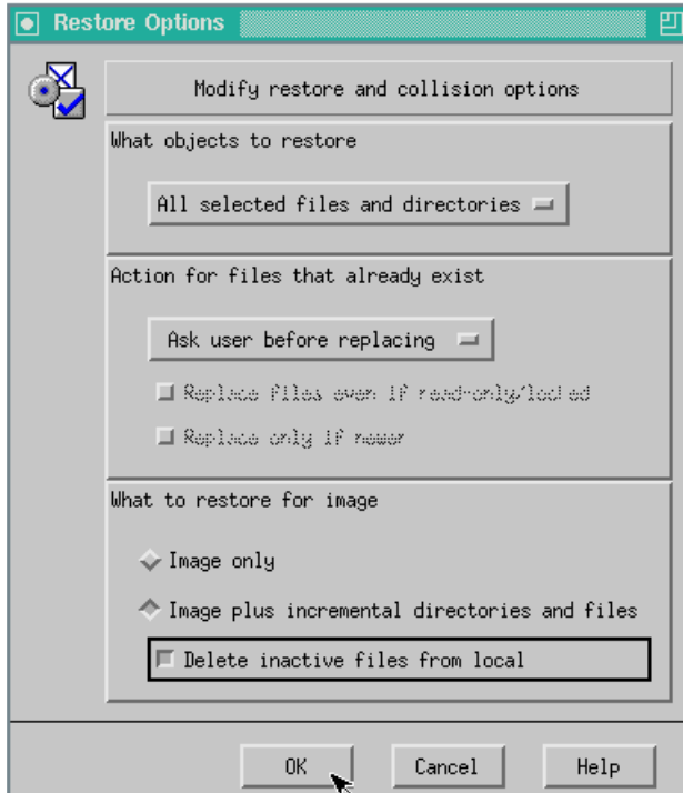
Figure 5-37 Chose whether to update the restored filesystem to a point in time
