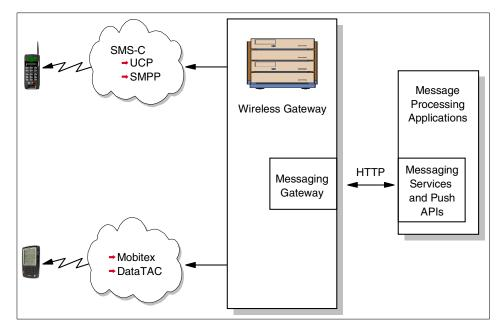
Figure 8-23 Messaging gateway accepting mobile-originated messages
