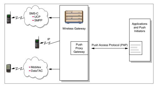
Figure 8-22 Wireless Gateway configured as a WAP push proxy gateway
