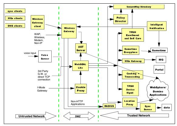
Figure 1-19 Deploying the Service Provider Offering
