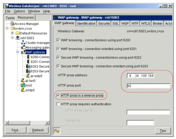
Figure 7-16 WAP Gateway with HTTP reverse proxy (WTE/WSL) configuration
