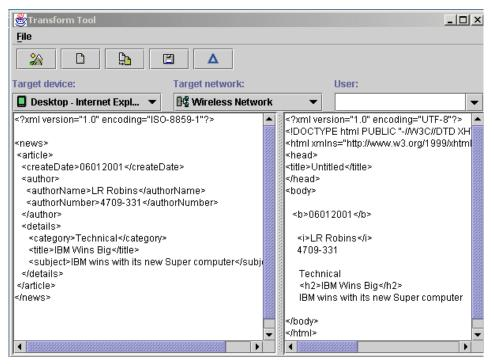
Figure 6-19 XSL Editor stylesheet results in the Transform Tool
