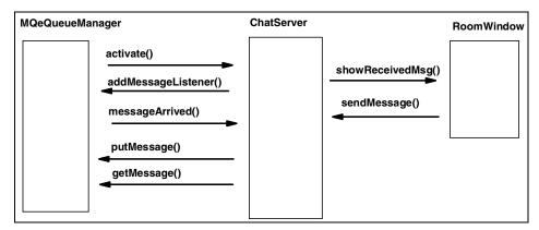
Figure 14-9 Class object interaction - server side
