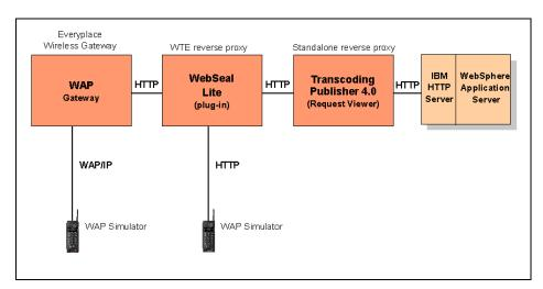
Figure 7-7 WML fragmentation with WebSphere Transcoding Publisher as a reverse proxy
