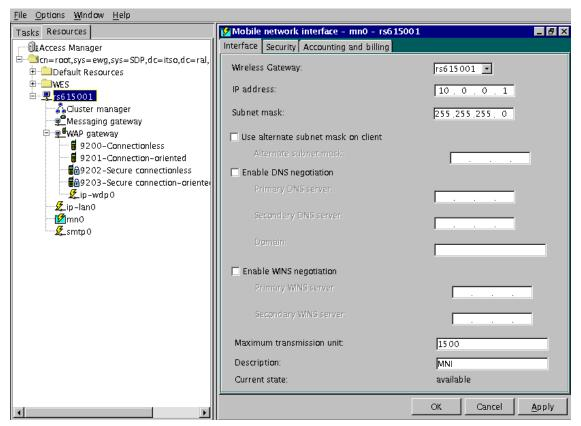
Figure 8-7 Sample MNI configuration using Everyplace Wireless Gateway Gatekeeper
