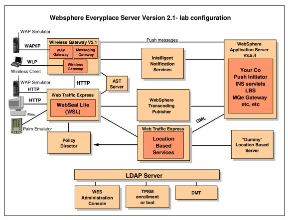
Figure 3-27 Lab configuration
