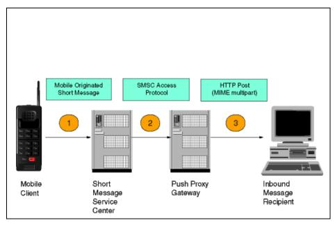
Figure 9-12 Receiving a mobile-originated Push
