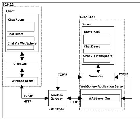
Figure 14-47 Incorporating the Wireless Gateway
