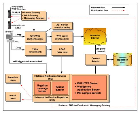
Figure 10-5 Request and notification flow in INS
