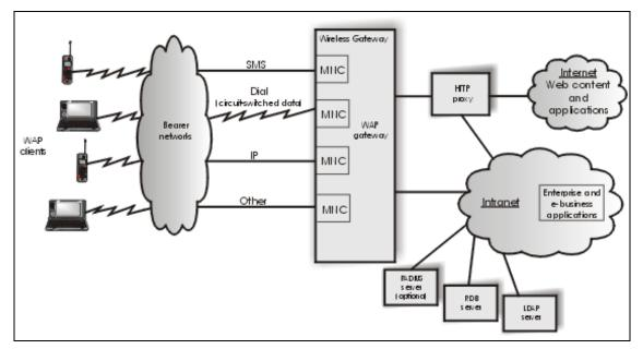
Figure 9-4 Wireless Gateway configured as a WAP gateway
