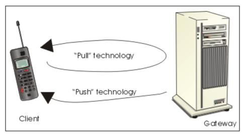
Figure 9-1 Simplified view of push versus pull operation
