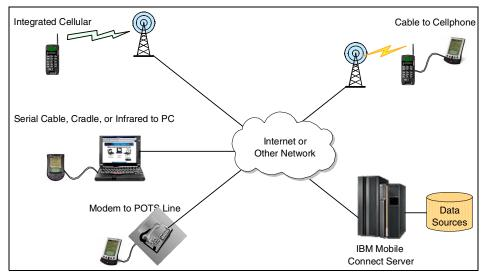
Figure 13-1 IBM Mobile Connect device connectivity
