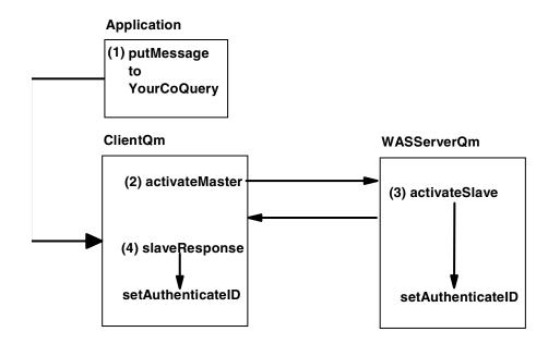
Figure 14-39 Authentication adapter flow
