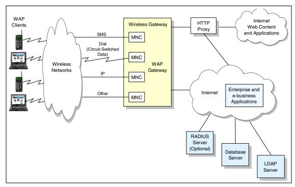
Figure 8-9 Wireless Gateway configured to include a WAP Gateway
