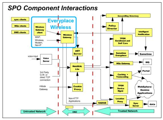
Figure 8-4 EWG interaction with the WebSphere Everyplace Server components
