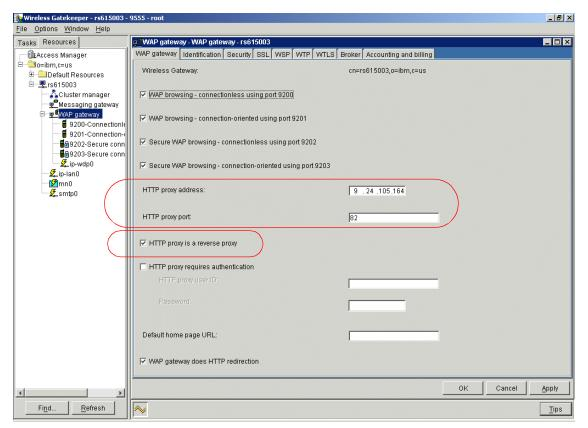
Figure 7-10 WAP Gateway configuration to connect to WTE/WSL reverse proxy
