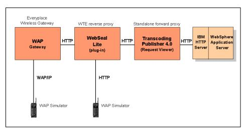
Figure 7-12 WML fragmentation with WebSphere Transcoding Publisher as forward proxy
