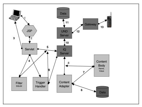
*Figure 10-15* Interactions between the individual components of the INS system for complex notification
