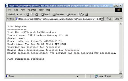
Figure 9-14 Results of push response from messaging gateway
