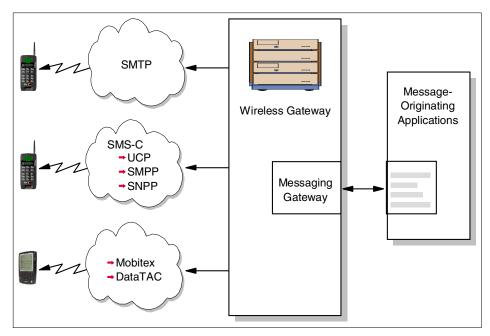
Figure 8-21 Wireless Gateway configured as a messaging gateway
