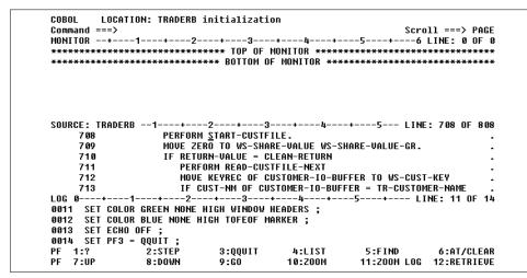
Figure 8-2 Debug Tool with a breakpoint set at START-CUSTFILE
