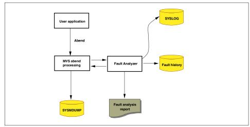
Figure 2-2 summarizes how Fault Analyzer works.
