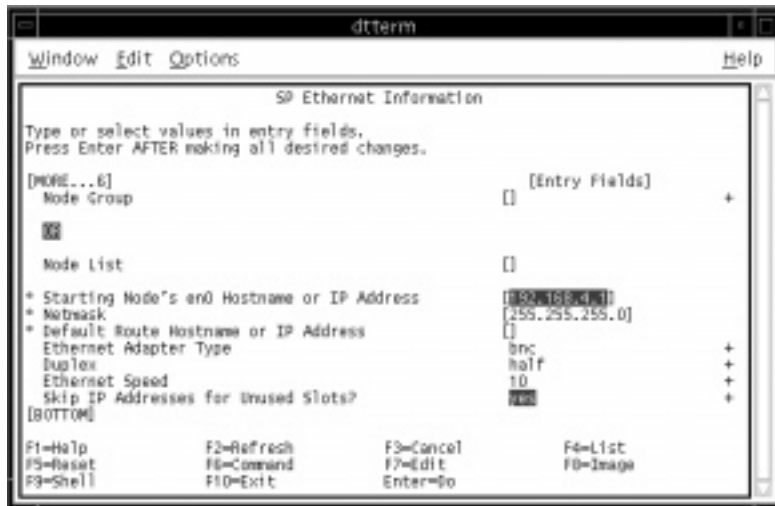
Figure 115. Setting Up The SP Ethernet Information
