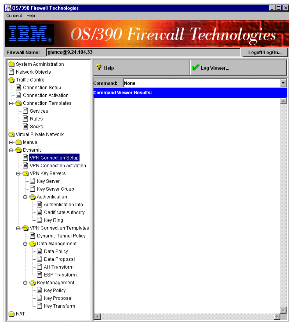
Figure 205. Firewall configuration client main screen - dynamic VPN definition
