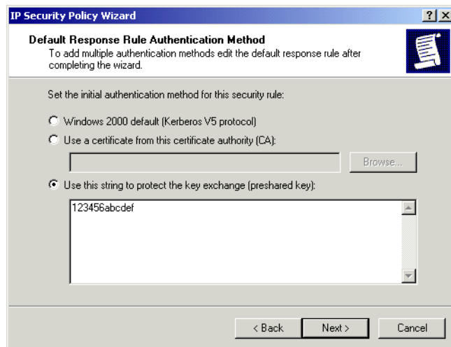
Figure 487. Windows 2000 - IPSec policy configuration: Default Response Rule Authentication Method
