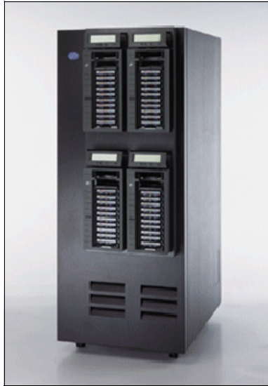
Figure 11-13 IBM TotalStorage Enterprise Tape Drive 3590 in a rack
