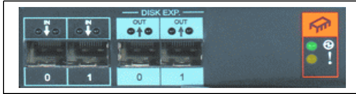
Figure 8-11 SBOD controller card
