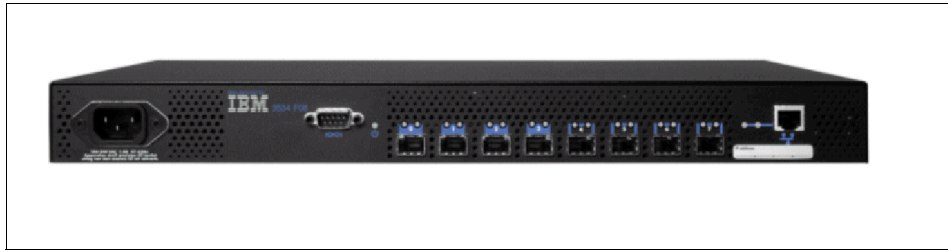
Figure 12-16 IBM SAN Fibre Channel Switch 3534-F08
