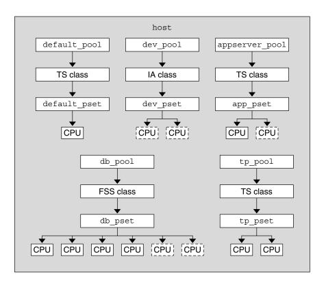
FIGURE 11–1 Server Consolidation Configuration
