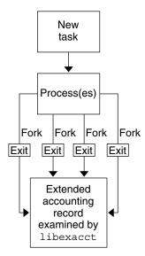
FIGURE 6-1 Task Tracking With Extended Accounting Activated
