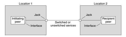
FIGURE 25–1 Parts of the PPP Link
