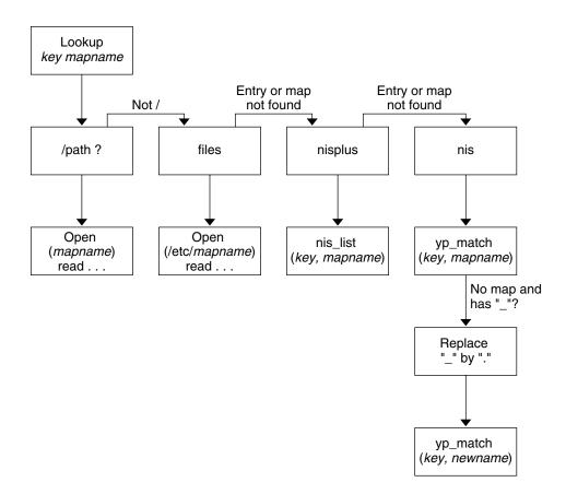
FIGURE 15-4 How Autofs Uses the Name Service
