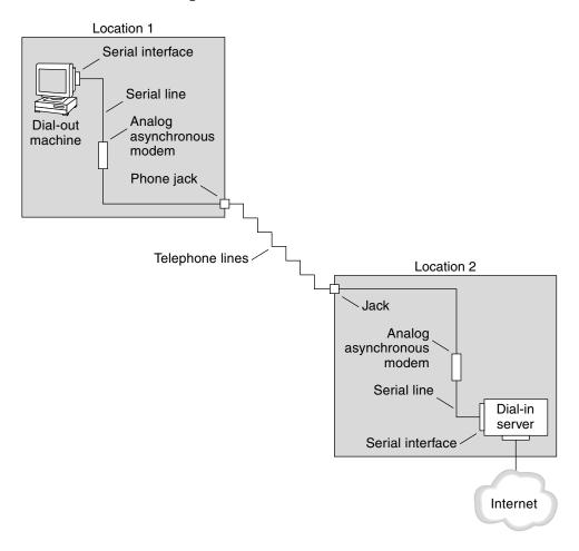
FIGURE 25-2 Basic Analog Dial-up PPP Link
