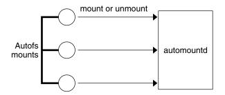
FIGURE 15-1 /etc/init.d/autofs Script Starts automount
