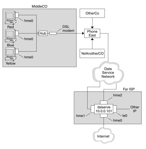
FIGURE 26–5 Example—PPPoE Tunnel
