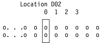
Figure 23. 6385 tape unit address jumpers for location D02
