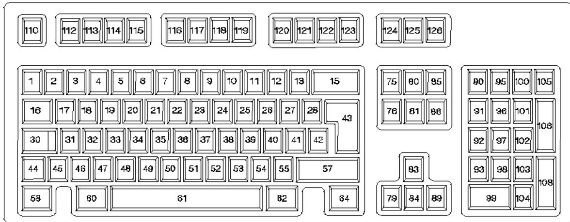
**Note:** The Swiss German and Swiss French variations of this keyboard are different in keyboard position codes 27, 40, and 41. In the following keyboard table these differences are indicated.
