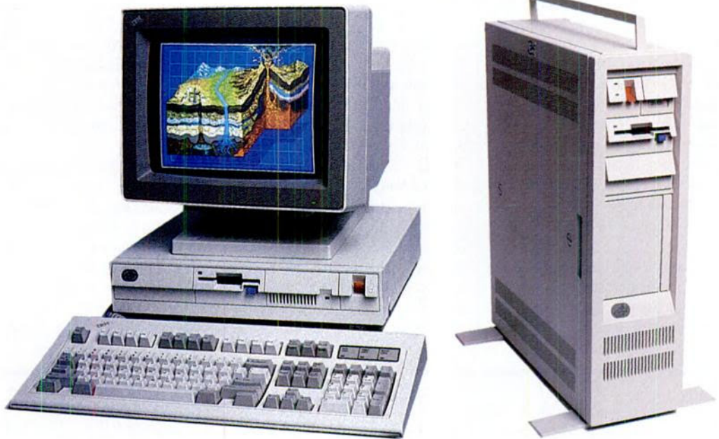
The Personal System/2 ranges from an 8086-based Model 30 (left), to the 80386-equipped Model 80. A line of four new analog displays—interchangeable among models—achieves higher resolutions and greater color choices than before.
