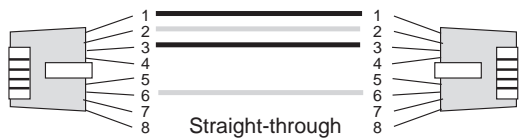
Figure 7. Straight-Through Network Cables
