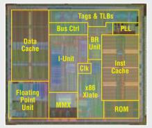
**OPTIMIZATION OF x86 ARCHITECTURE.** The IDT WinChip is fully compatible with, and optimized for, x86 architecture in industry-standard Socket 7, enabling direct installation in existing designs and future upgrades.
