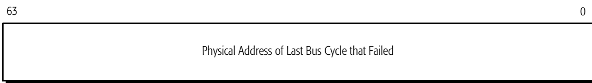
Figure 1-8. Machine-Check Address Register (MCAR)
