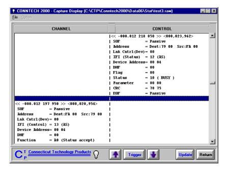
The **Analyzer** displays the Captured data in a format that is both easy to read and understand. Each frame is time stamped relative to the Trigger Point. The number of idles between frames is also displayed. The example above shows Control Unit Status being reported to the Channel. Samples Captures and Trigger Settings are furnished with the software.
