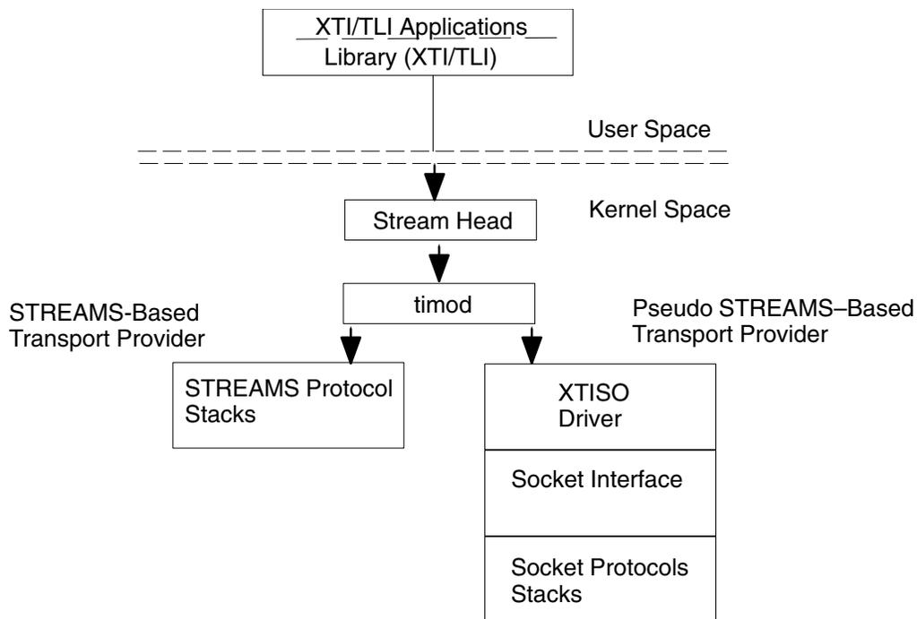
Figure 1. . This illustration shows the implementation of XTI/TLI with STREAMS. It shows that the X/Open Transport Interface (XTI) Stream, in user space, always consists of a Stream head, in kernel space, and the transport interface module, **timod**. Depending on the transport provider specified by the application, **timod** accesses either the STREAMS-based protocol stack natively or a socket-based protocol through the pseudo-driver, **xtiso**
