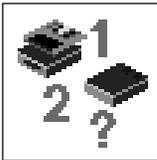
**Multi-Boot:** Enables you to set and view the default operating system, modify the boot sequence, access the Open Firmware command prompt, and other options.
