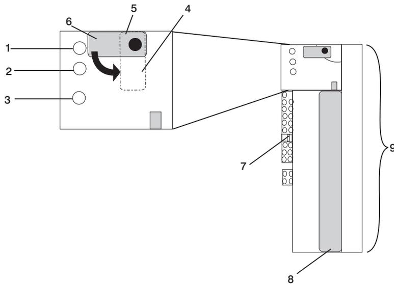
Figure 4. Installing the 10,000 RPM SSA Hot-Swap Disk Drive
