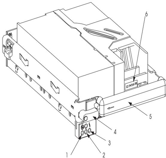
Figure 1. 7200 RPM SSA Hot-Swap Disk Drive
