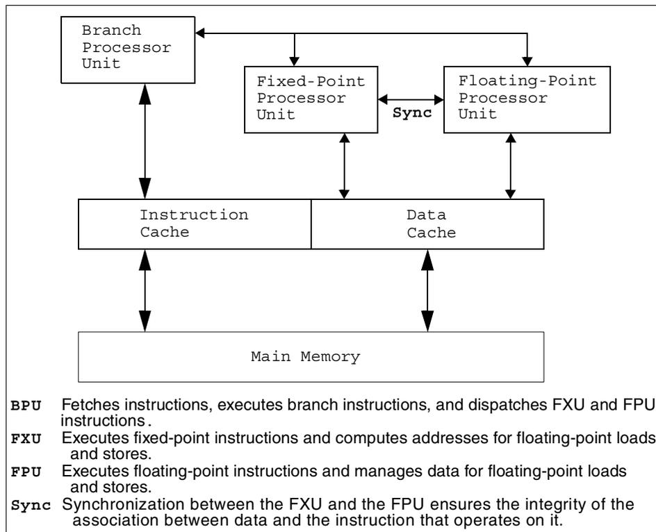
Figure 2. Pipelined Architecture
