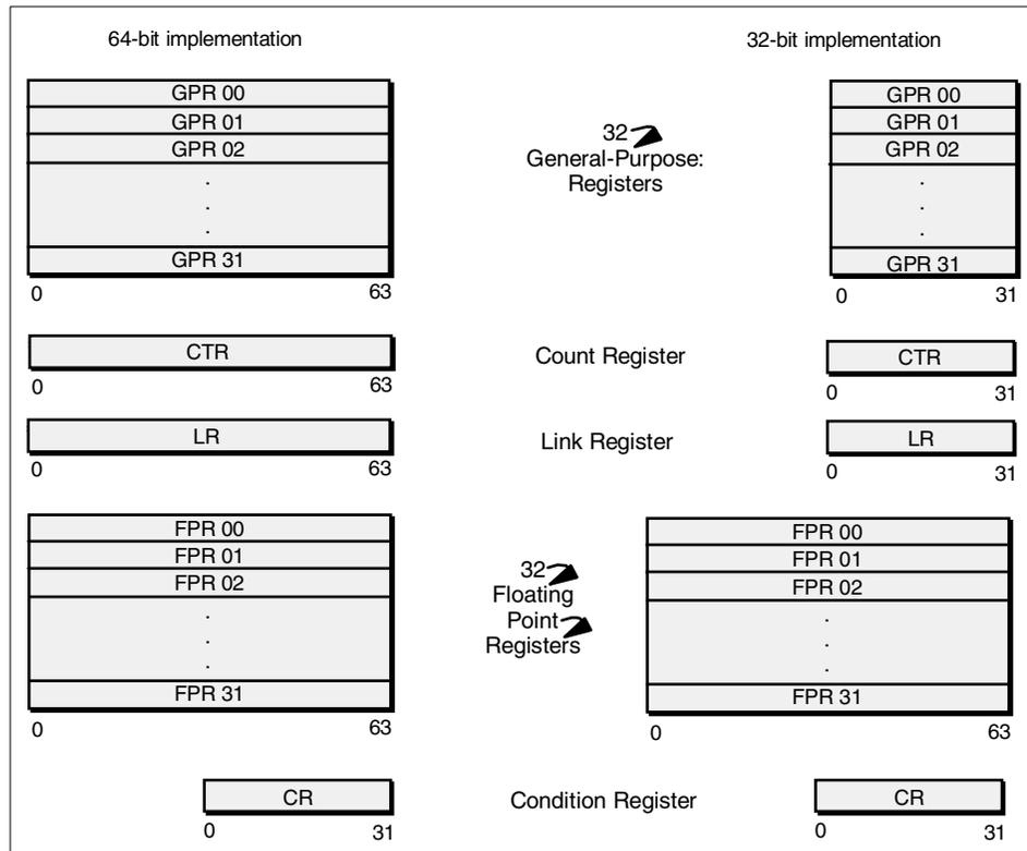
Figure 11. Register Implementation of 32 and 64-bit PowerPC Processors
