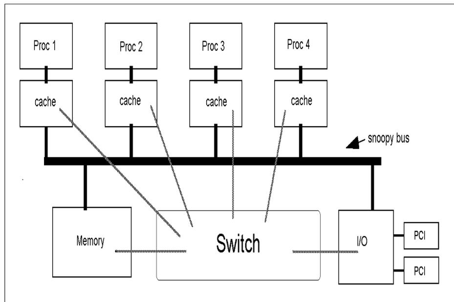
Figure 29. Using a switch for data transfers
