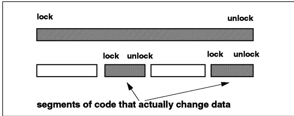
Figure 32. Lock Granularity
