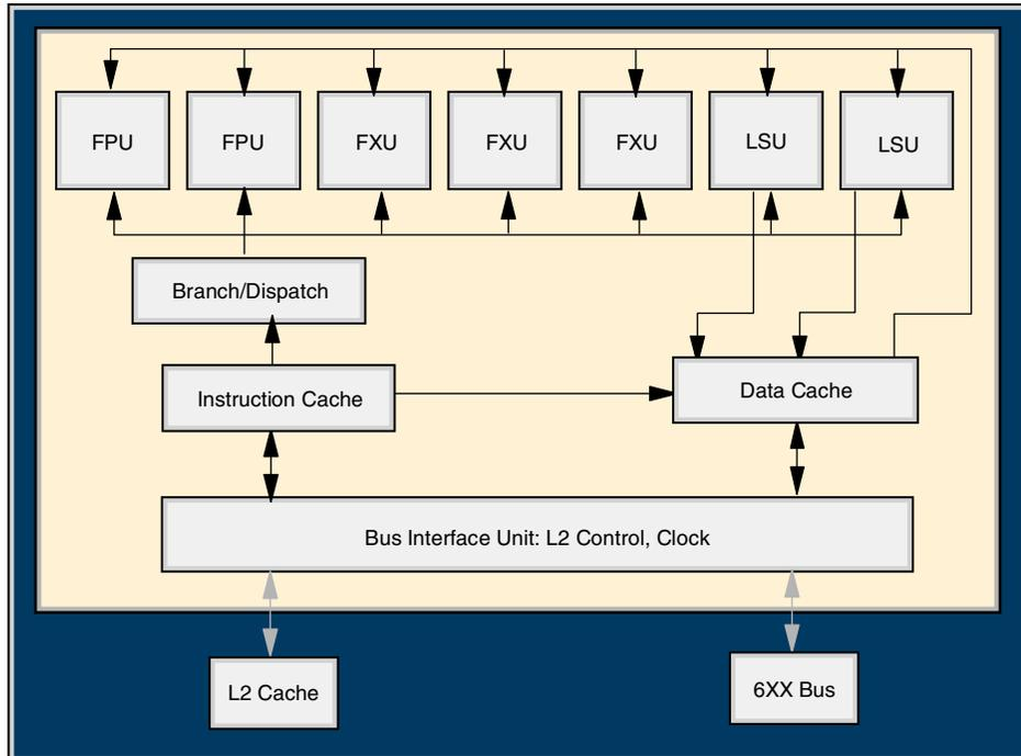
Figure 16. POWER3 II Processor
