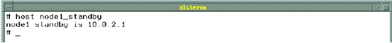
A terminal window titled 'aixterm' with a green header bar. The terminal shows the command 'host node1\_standby' and its output: 'node1 standby is 10.0.2.1'. The prompt is '# \_'.
