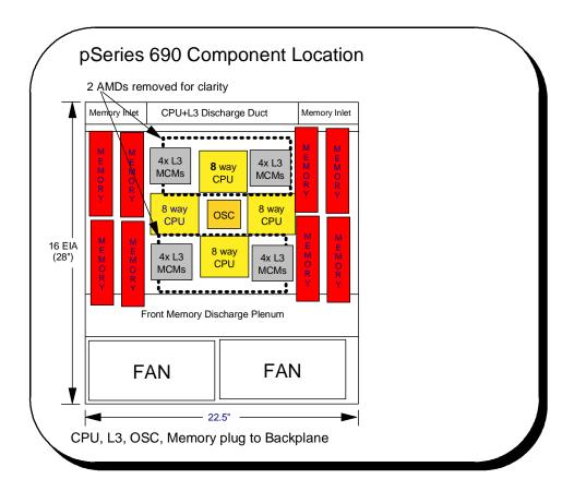
We use the term Air Moving Device (AMD) as a generic term for either a fan or a blower. Variable speed AMDs in the system unit along with variable speed AMDs in the I/O units allow for increased air flow to maintain proper cooling levels in case of an AMD fault.
