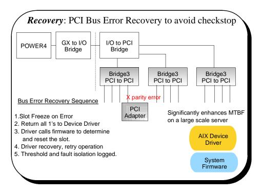
To support this, AIX device drivers must be written to a standard called EEH enabled, which requires that they respond to a special data packet generated from the affected PCI slot hardware by calling system firmware which will examine the affected bus, and allow the device driver to reset it, and continue. For maximum system availability and recovery, IBM recommends that only EEH enabled PCI adapters be used.
