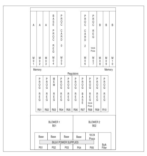
Figure 18. Front view of the pSeries 680 and S80 CEC
