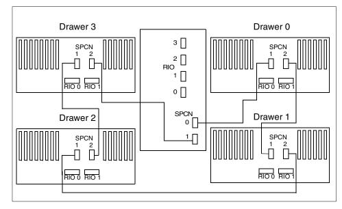
Figure 6. Fully configured SPCN loop with four I/O Drawers
