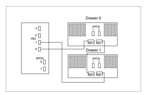
Figure 8. One RIO loop attached to two I/O Drawers
