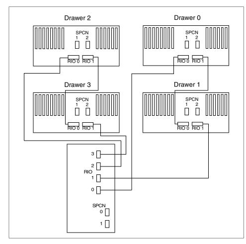
Figure 10. Two RIO loops attached to four I/O Drawers
