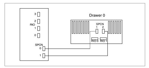
Figure 5. Base SPCN loop with one I/O Drawer
