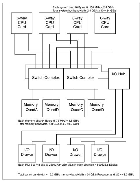
Figure 23. System switch complex
