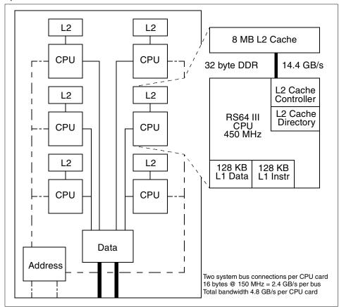
Both are 64-bit, PowerPC-compatible, four-way superscalar implementations optimized for commercial workloads.
