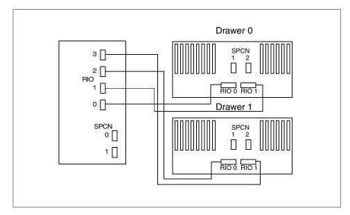
Figure 9. Two RIO loops attached to two I/O Drawers
