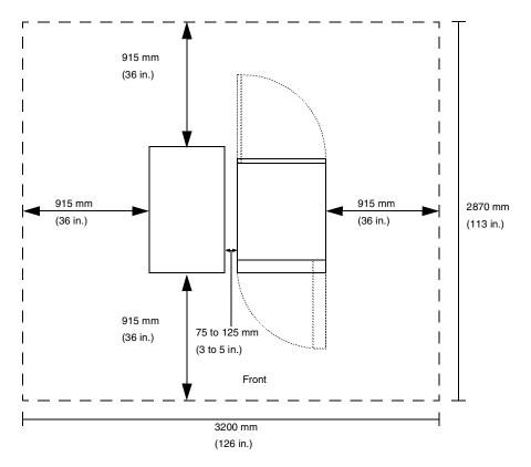
Figure 28. pSeries 680 and S80 system service clearances
