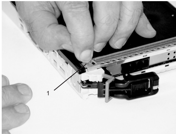
1 Location of the Installed Bushing and Bushing-Lock Pin
