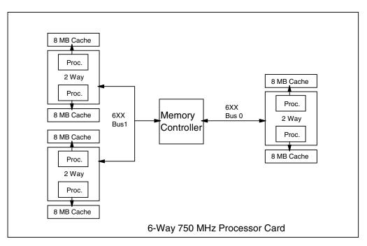
Figure 4. pSeries 660 Model 6H1 System Schematic for 6-Way Processor 750 MHz
