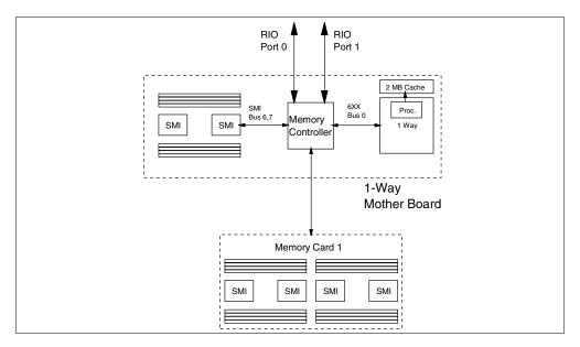
Figure 3. Model 6H1 System Schematic for 1-Way Processor within the CEC
