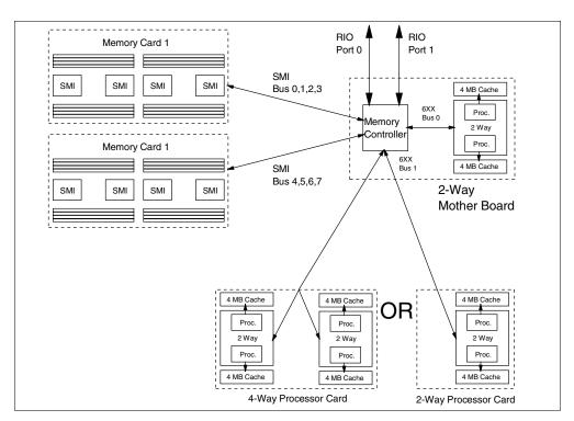
Figure 2. Model 6H1 System Schematic for 2-, 4-, or 6-Way 600 or 668 MHz SMP within the CEC
