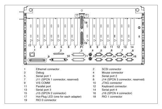
Figure 5. I/O Drawer Rear View
