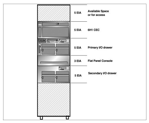
Figure 1. Model 6H1 with Two I/O Drawers and Flat Panel Console in a T00 Rack
