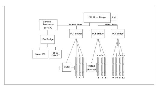
Figure 8. Internal Architecture of Model 6F1
