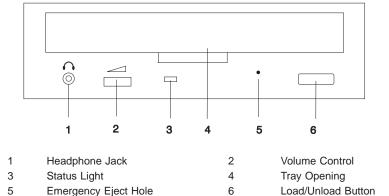
When the CD-ROM is set to On, the status light (3) indicates one of several conditions. The following are status light states and the respective conditions of the CD-ROM drive:
