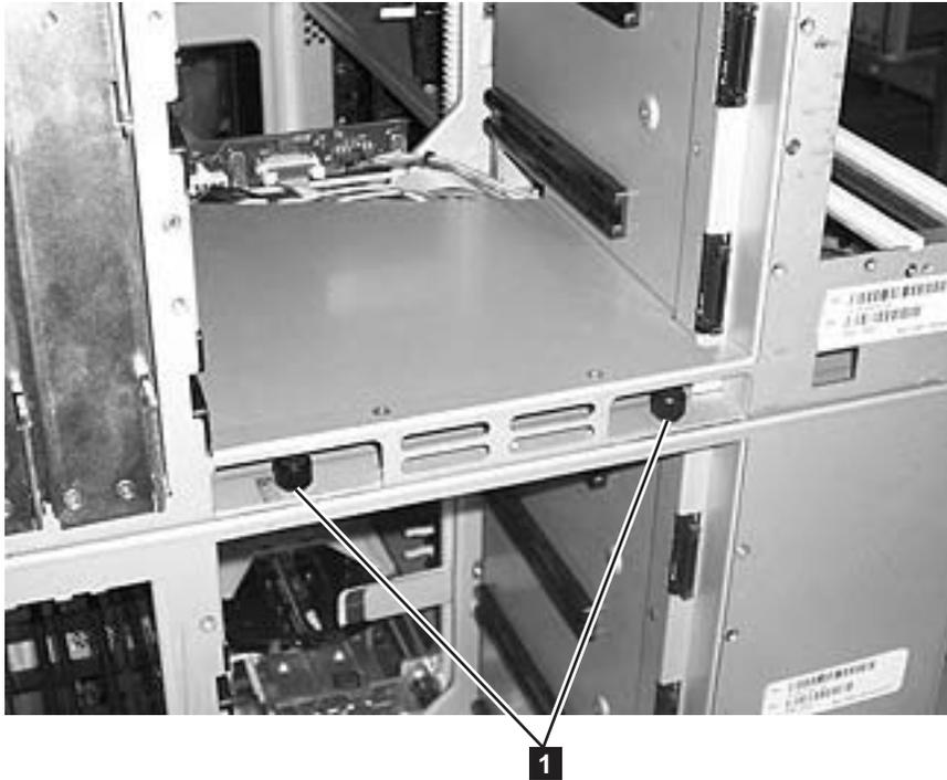
Figure 8-7. Control module rear thumb screws
