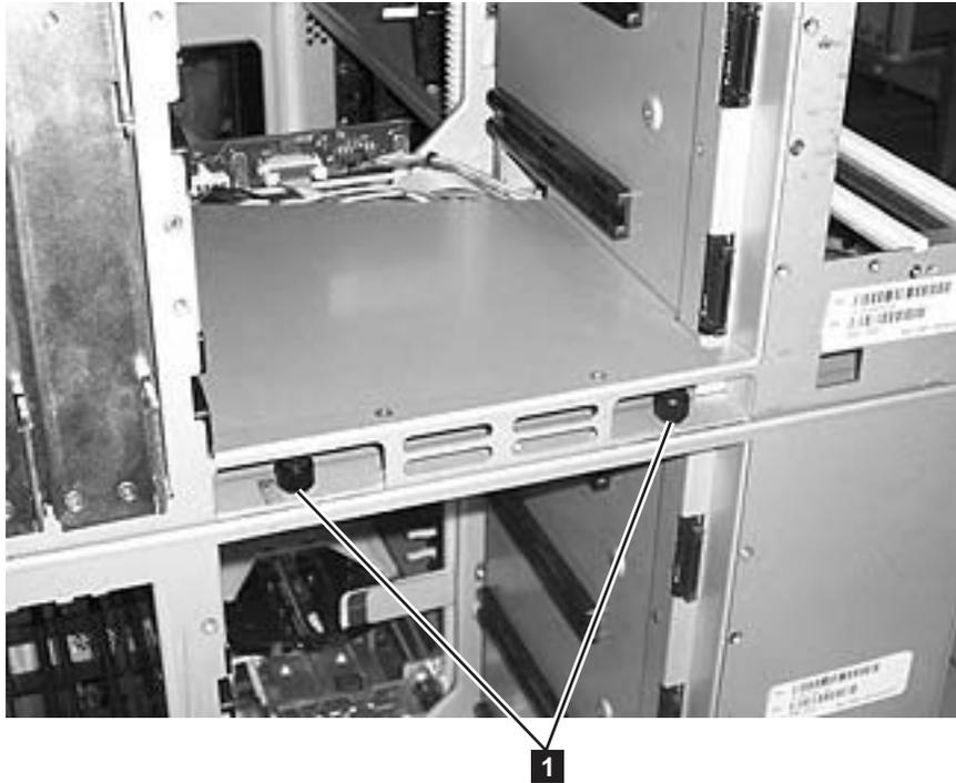
Figure 8-3. Control module rear thumb screws
