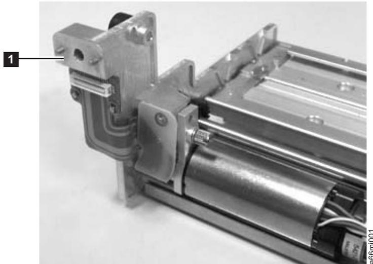
Figure 8-35. Thumbscrew securing Cable Spool
