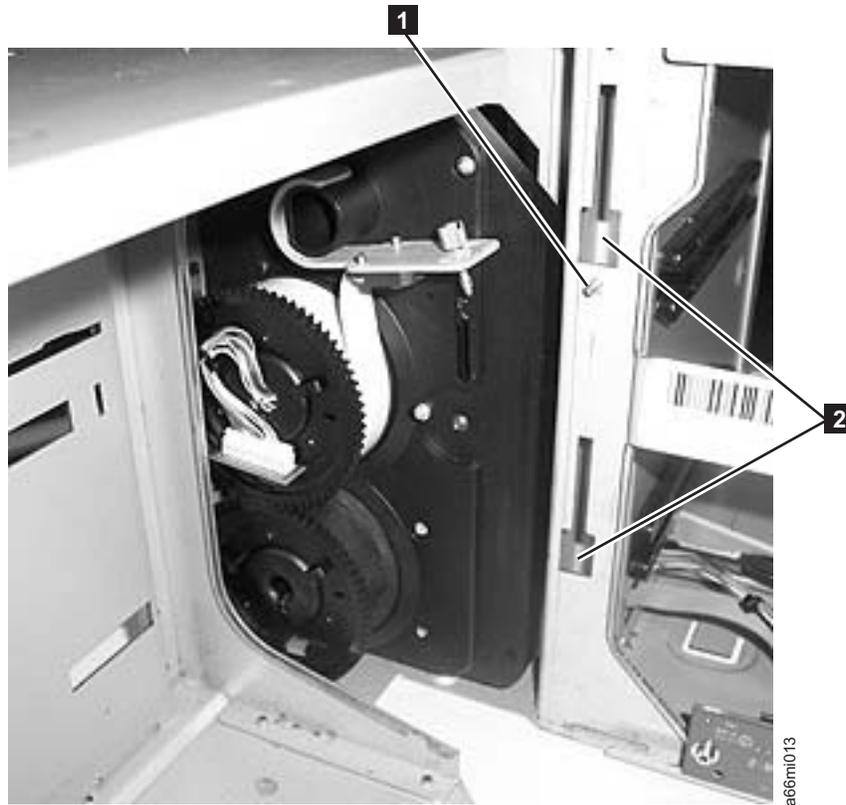
Figure 8-60. Rear gear rack location on chassis
