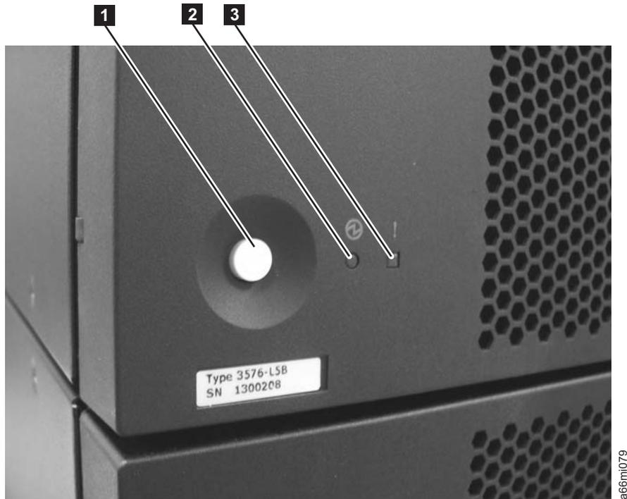
Figure 7-1. Power button LEDs
