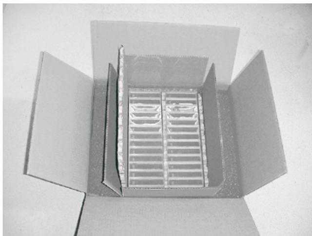
Figure 5-6. Double-boxing tape cartridges for shipping
